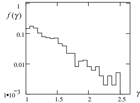
**Fig. 4.** Energy distribution function of electrons in the fields of waves  $H_{11}$  and  $H_{21}$  at  $t = 200\pi$ .
