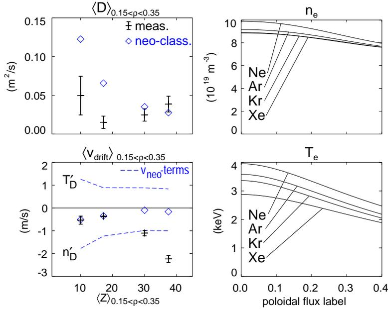
**Figure 4.** Line averaged diffusion coefficient  $\langle D \rangle$  and drift velocity  $\langle v_{drift} \rangle$  for the range of poloidal flux labels  $0.15 < \rho_{pol} < 0.35$  versus impurity charge  $\langle Z \rangle$  in the same radial range. The measured transport parameter are compared with results from neo-classical calculations ( $\diamond$ ). The density and temperature profiles for the calculations are shown on the right side.
