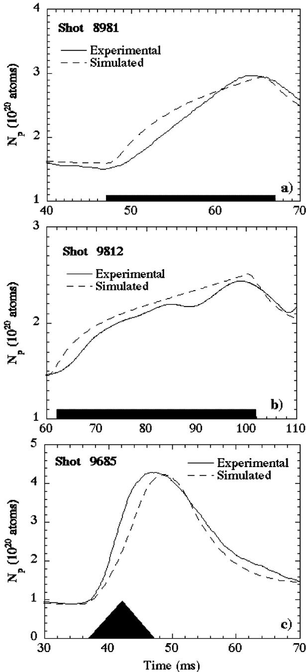
**Figure 1:** 0-dimensional simulations of three RFX discharges perturbed by gas puffing. The additional influxes are indicated by the shadowed areas.
