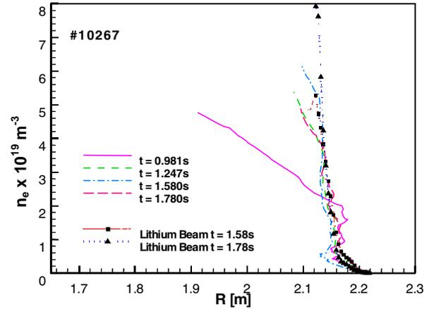
**Fig. 1** Reflectometry density profiles measured at the OH ( $t = 0.981$ s), L ( $1.274$ s) and H-phases (quiescent:  $1.58$ s, and between ELMs:  $1.78$ s) for #10267. Li-Beam measurements are shown also for  $t = 1.58$ s,  $1.78$ s.
