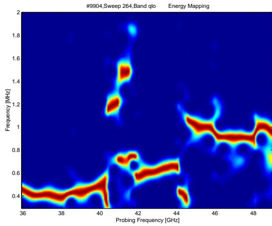
**Fig. 4** Time-frequency distribution of the reflected signal ( $Q$ -band channel:  $33\text{--}50 \text{ GHz}$ ), for the case of Fig.3.
