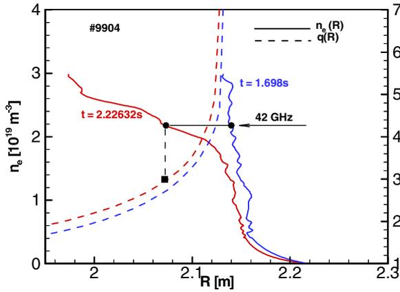
**Fig. 3** Density profiles obtained from broadband reflectometry, at  $t = 1.698s$  and  $2.226s$ . The location of the density layer probed by the fluctuations monitor ( $42 \text{ GHz} \Leftrightarrow 2.19 \times 10^{19} \text{ m}^{-3}$ ), is indicated, both in  $n_e$  and  $q(r)$ .
