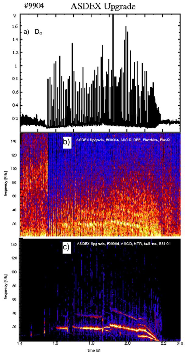
**Fig. 2** a) Magnetic signal from a pick-up coil; b) Time evolution from FFT power spectra of the reflectometry signals; c) time evolution of magnetic fluctuations frequency data
