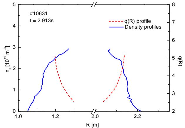
Fig. 6 Density and  $q$  profiles for the case of Fig. 5 ( $t = 2.913s$ , #10631)
