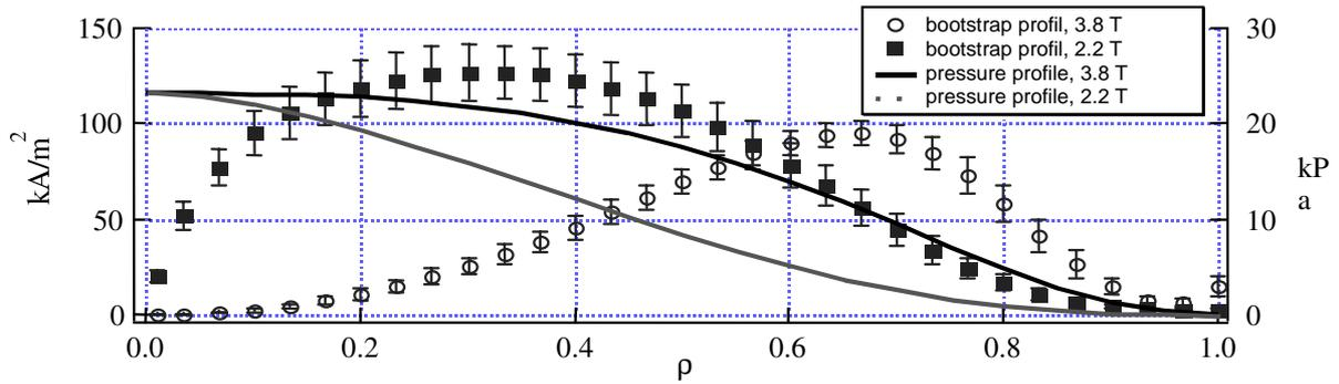
**Figure II-2 :** bootstrap profiles (markers) for two different magnetic fields (lines → pressure profile). The error bars are due to errors on experimental data (Temperature, density,  $q$  profile)
