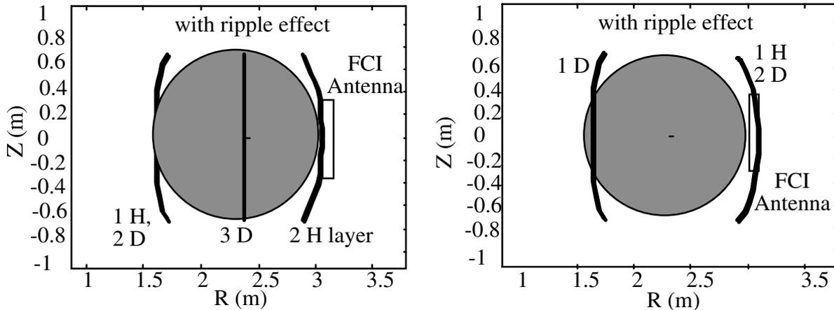
**Figure I a)** FWEH scheme at  $B_0 = 2.1 \text{ T}$ ,  $R_0 = 2.28\text{m}$ ,  $a = 0.71 \text{ m}$  (shot 18805).
