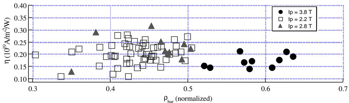
**Figure II-5 :** Current drive efficiency of FWEH for stationary shots in a large set of plasma parameters
