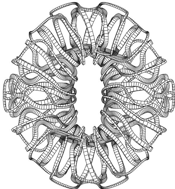
**Fig. 3.** Modular coil system for a quasi-axisymmetric tokamak [6]: set of main coils with  $N_c = 12$  coils per period, set of auxiliary coils with  $N_{\text{aux}} = 8$  coils per period. Number of periods  $N_p = 2$
