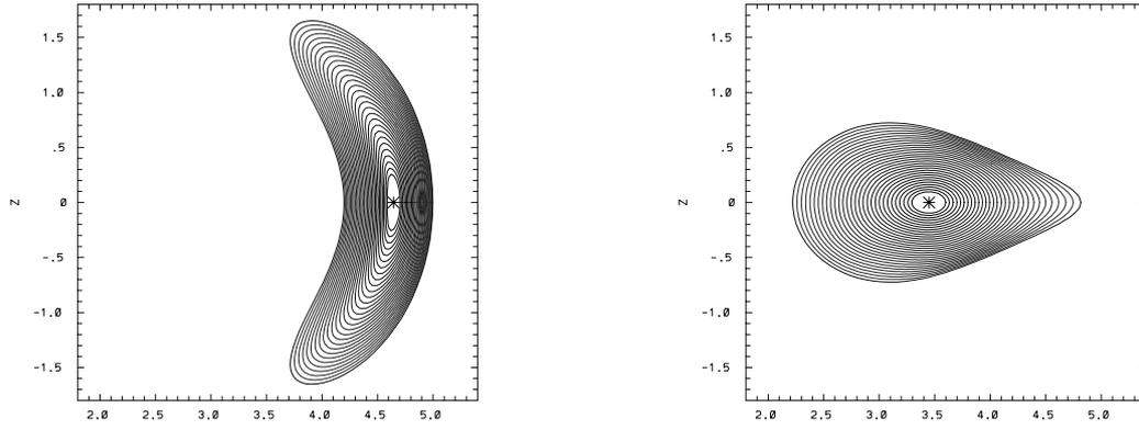
**Fig. 1.** Fixed-boundary equilibrium of a quasi-axisymmetric tokamak configuration: Aspect ratio  $A \approx 4$ ,  $\langle \beta \rangle \approx .03$ , rotational transform  $\iota \approx 0.51$ (axis),  $0.56$ (edge), toroidal plasma current  $I_{\text{tor}} = -0.015 \cdot I_{\text{pol}}$ ,  $I_{\text{pol}} = \text{coil current}$
