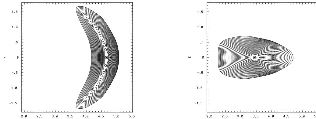
**Fig. 2.** Free-boundary equilibrium of the above case obtained in the external field of the main coil set. The coils (Fig.3) are determined such that the plasma configuration, defined in Fig.1, is reproduced.
