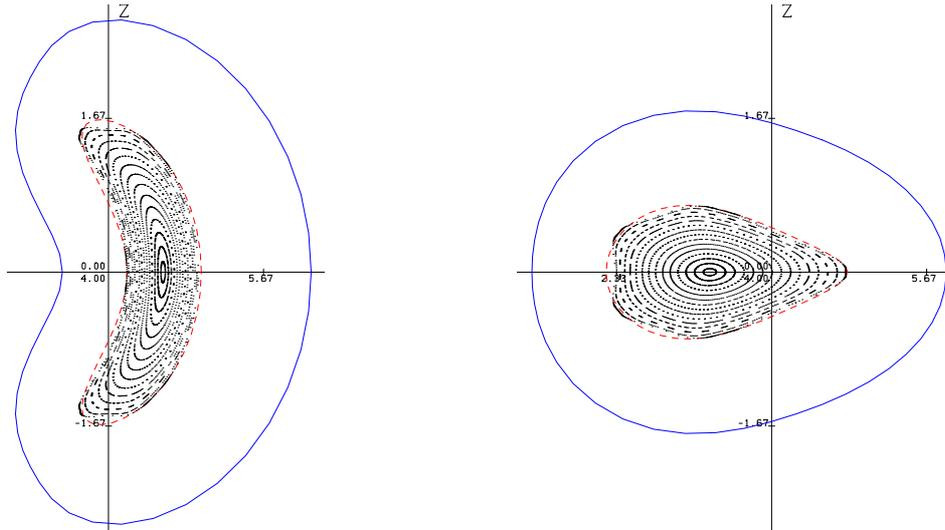
**Fig. 4.** Poincaré plots of the vacuum field produced by the coil system with  $I_{\text{aux}} = -0.16 \cdot I_{\text{pol}}$ . Boundary (red) of the quasi-axisymmetric tokamak, filament carrying surface (blue)
