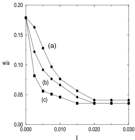
Fig.2 The saturated island width versus  $I=I/I_p$ , the relative amplitude of the driven current. Curve (a) is obtained with  $\Delta\eta=0$ , curve (b) with  $\Delta\eta=0.05$ , and curve (c) with  $\Delta\eta=0.1$ .
