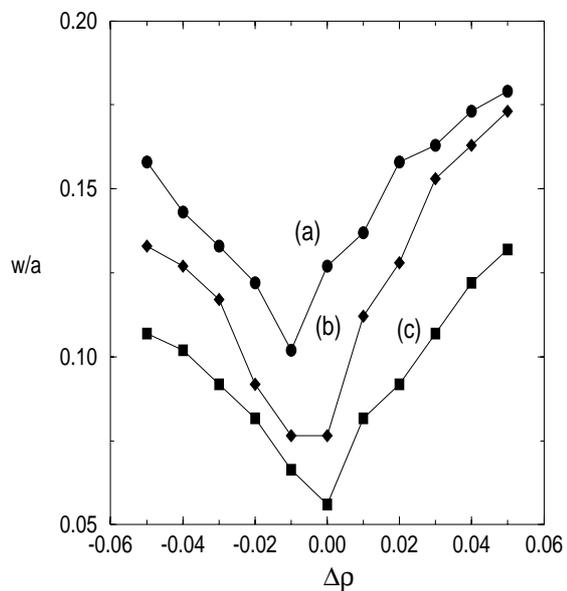
Fig.4 The saturated island width versus  $\Delta\rho=(r_E-r_S)/a$ . Curve (a) is obtained with  $I=0.005$  and  $\Delta\eta=0.0$ , curve (b) with  $I=0.01$  and  $\Delta\eta=0.0$ , and curve (c) with  $I=0.005$  and  $\Delta\eta=0.1$ .
