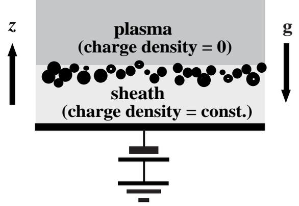
Figure 5. Plasma, sheath, and dusts near plane electrode.
