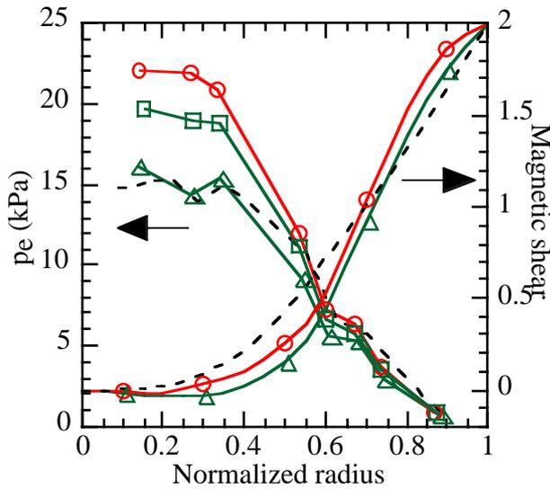
Figure 6: Electron pressure and magnetic shear profiles of shot #TS25196 in Fig 3, at  $t = 9.8$  s (triangle, 2MW),  $t = 10.2$  s (square, 4MW), and  $t = 10.8$  s (circle, 4MW). Dashed curve corresponds to the reference L-mode shot.
