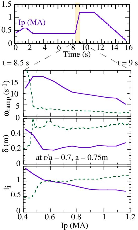
Figure 1: Ramp-up rate, skin depth (at  $r/a = 0.7$ ), and self-inductance versus total current for two scenarios. Case 1 (full): ramp-up between 8.5 s and 9 s, after a steady-state  $I_p = 0.4$  MA. Case 2 (dashed): start-up phase between 0.1 s and 2.5 s.
