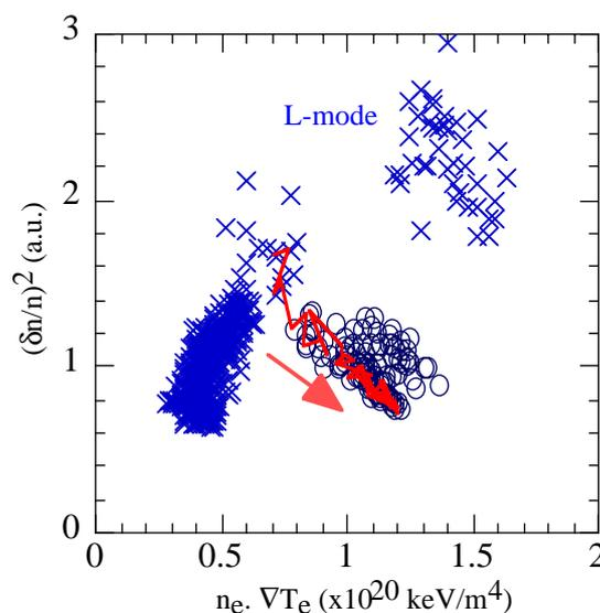
Figure 9: Statistical analysis of density fluctuation versus  $n_e \cdot \nabla T_e$ . Cross: L-mode. Circle: shots of scenario described in this paper, the full line illustrates the trajectory of one of these shots.
