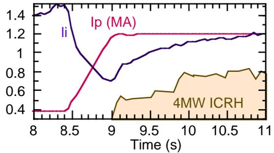
Figure 3: ICRF H-minority heating discharge with preformed hollow current profile.
