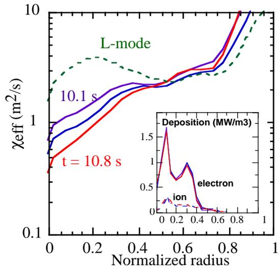
Figure 7: Comparison of 1-Fluid effective diffusivity (#TS25196) with a reference L-mode.
