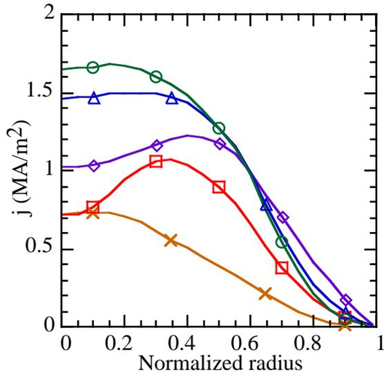
Figure 4: Current profiles of discharge #TS25196, in Fig 3, before (at  $t = 8.2$  s: cross, and  $t = 8.7$  s: square) and after ICRF application (at  $t = 9.1$  s: diamond,  $t = 9.8$  s: triangle,  $t = 10.8$  s: circle).
