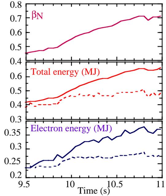
Figure 5: Time evolution normalized beta ( $\beta_N$ ), total and electron energies (dashed curves correspond to the ITER L-mode scaling for total energy and the electron Rebut-Lallia-Watkins L-mode scaling).
