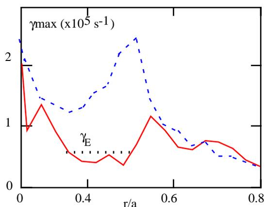
Figure 8: Radial profile of linear growth rate for shot #TS25196, at  $t = 9.1$  s. Dashed curve: calculation assuming a monotonic  $q$  profile. Stabilizing ExB shear is from neoclassical calculation with the ripple effect.
