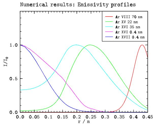
**Fig. 2:** Radial profiles of normalized argon emissivities calculated by STRAHL for TEXTOR #80664 ( $T_e(0) = 1.6$  keV,  $n_e(0) = 4.5 \times 10^{13} \text{ cm}^{-3}$ )
