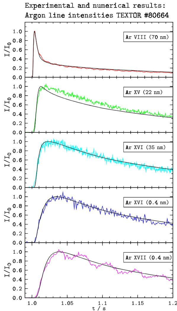
**Fig. 1:** Measured line intensities (coloured lines) and STRAHL results (black solid lines) for TEXTOR #80664
