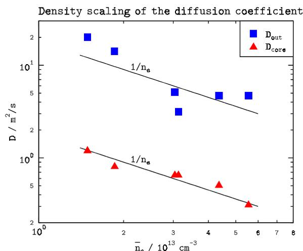
**Fig. 4:** Scaling of the diffusion coefficient with mean electron density for constant current  $I = 330$  kA and NBI heating power  $p = 1.34$  MW
