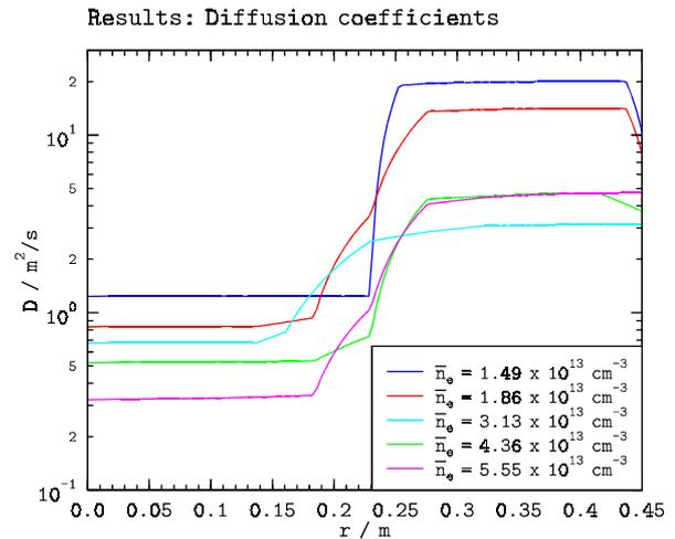
**Fig. 3:** Radial profiles of diffusion coefficients ( $I = 330$  kA,  $B = 2.25$  T, NBI power  $p = 1.34$  MW)
