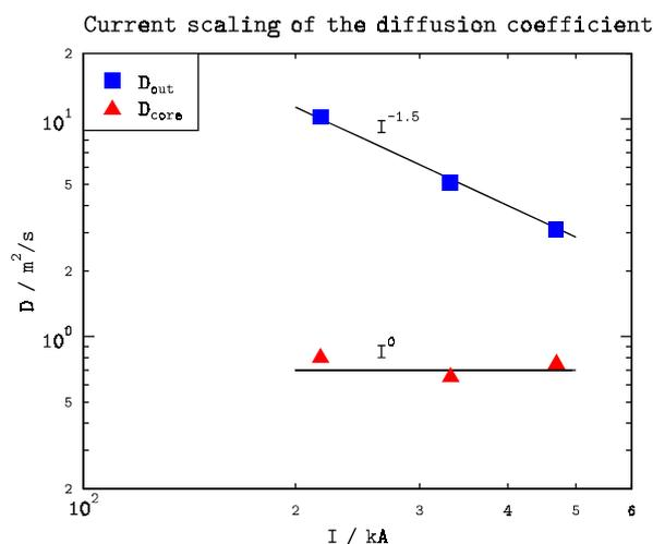
**Fig. 5:** Scaling of the diffusion coefficient with plasma current at constant electron density  $\bar{n}_e = 3 \times 10^{13}$  cm<sup>-3</sup> and NBI heating power
