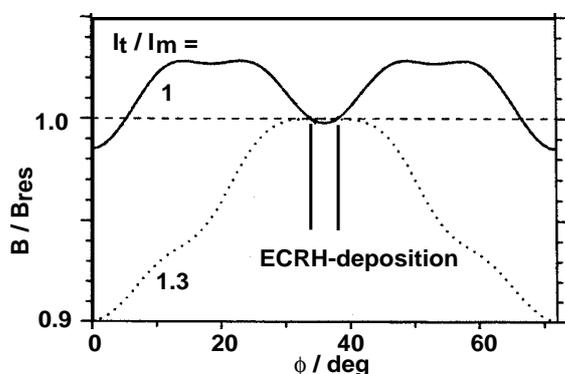
Fig. 4: Example for relative magnetic field strength on axis within one field period for standard configuration ( $I_t/I_m=1$ , solid line) and  $B_{max}$ -configuration ( $I_t/I_m = 1.3$ , dotted line).
