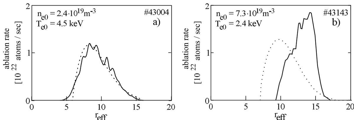
Fig.5: Comparison of ablation rate profiles deduced from the measured CII-line emission (solid lines) and those calculated by the NGS model (dotted lines): a) „B<sub>max</sub>“-configuration and b) standard-configuration.
