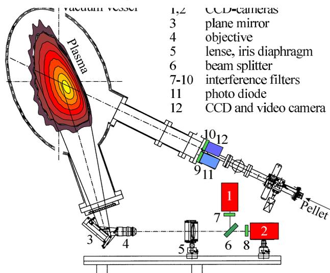
Fig.1 : Injection geometry at W7-AS and experimental instrumentation for pellet observation
