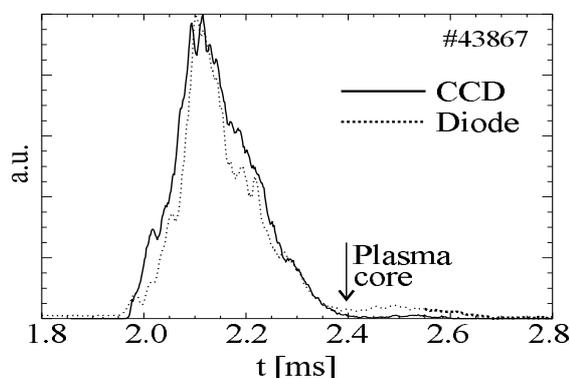
Fig.3: Temporal evolutions of CII emission measured by the diode and CCD camera 2.
