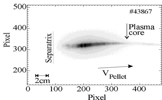
Fig.2: Pellet trajectory as seen from CCD camera 2 behind CII-filter, integrated over the pellet lifetime. Locations of separatrix and plasma center are marked
