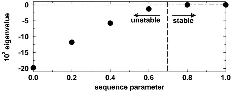
FIG. 4: Result of a global ideal MHD stability study of the  $\langle\beta\rangle = 4\%$  equilibrium: CAS3D2 eigenvalues versus an artificially introduced factor which was applied to the main stabilizing term in the MHD energy functional, so that for sequence parameter unity the full MHD energy functional is obtained. The stability limit is reached at approximately 0.7 in the sequence parameter.
