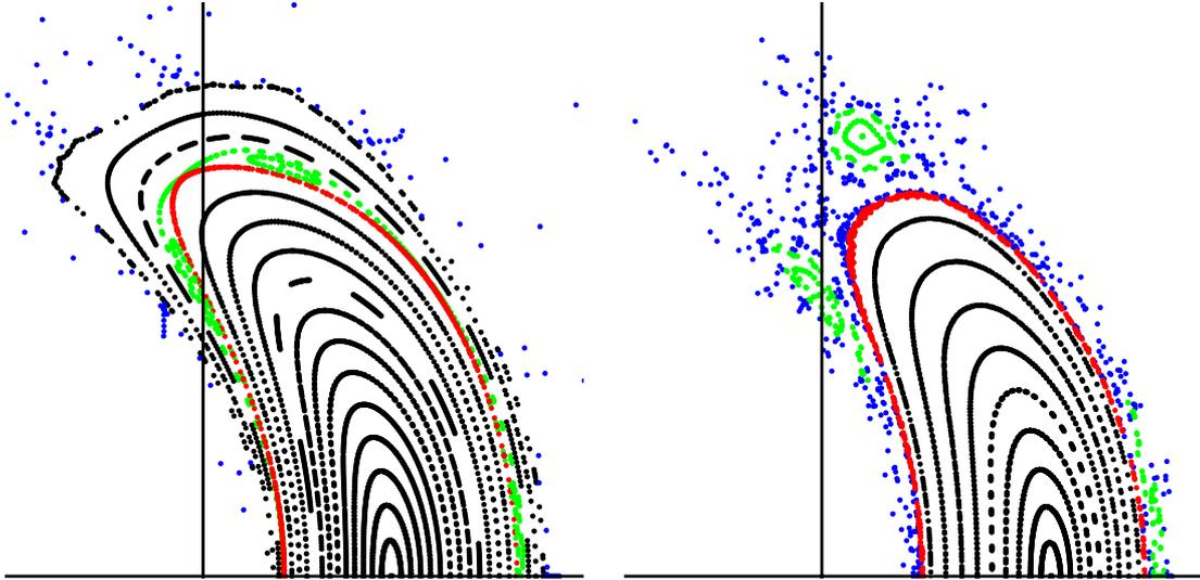
FIG. 1: Upper halves of the Poincaré plots at the symmetric bean-shaped cross-section for the vacuum magnetic field (left figure) and the finite- $\beta$  magnetic field with  $\langle\beta\rangle = 4\%$  (right figure).
