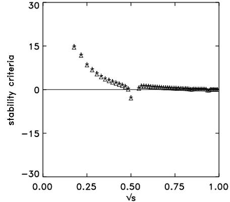
FIG. 3: Mercier (+) and resistive interchange ( $\Delta$ ) criteria versus  $\sqrt{s}$  for  $\langle\beta\rangle = 5\%$ . Instability occurs at  $\sqrt{s} \approx 0.5$  for  $\iota = 5/6$ .
