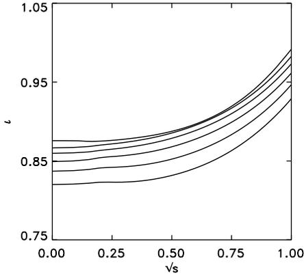
FIG. 2: Rotational transform profiles  $\iota$  for the vacuum field (upper curve) and the finite- $\beta$  magnetic fields up to  $\langle\beta\rangle = 5\%$  (lower curve) versus  $\sqrt{s}$  with  $s$  the normalized flux label.
