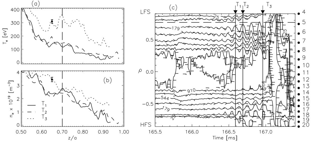
Figure 2: (a)  $T_e$  and (b)  $n_e$  high resolution TS temperature profiles measured at the indicated times in (c). Only the profile around  $q = 2$  is shown. For clarity just one typical error bar is shown. The vertical dashed line indicates the calculated radial position of the  $q = 2$  surface. (c) Time evolution of the radial temperature profile measured from the ECE radiometer. The channel numbers and its positions are indicated at the right.
