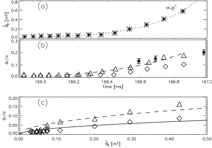
Figure 1: (a)  $\tilde{B}_\theta$ , (b)  $\Delta r/a$ . The three black circles indicate the island width estimated from the TS (see Fig. 2(a)). (c)  $\Delta r/a$  plotted against  $\tilde{B}_\theta$ . The symbols  $\Delta$  ( $\diamond$ ), refer to the low field side (high field side).
