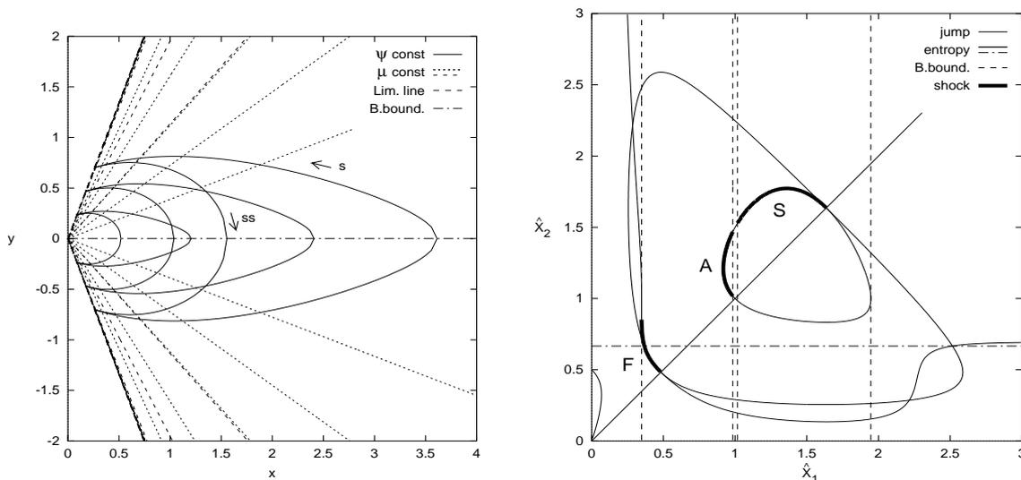
Figure 2: (a) Flow ‘reflected’ by the limiting line. (b) Fast, Alfvén, and slow shocks.
