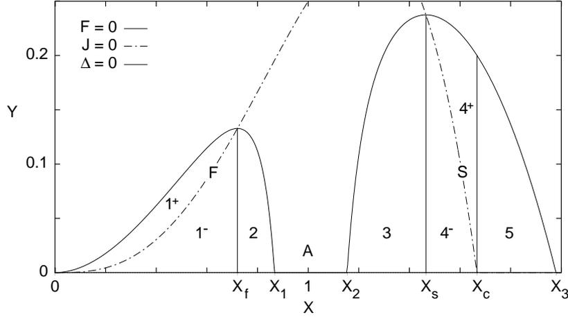
Figure 1: Four main flow domains due to the Alfvén gap & fast and slow limiting lines.
