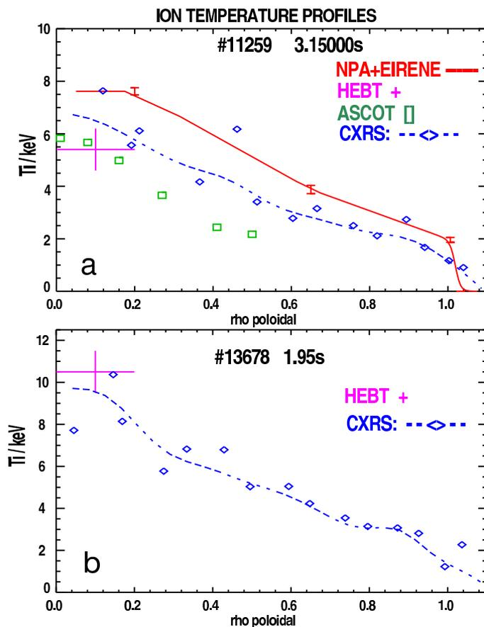
Figure 3 a,b: Ion temperatures from ASCOT Simulations, CXRS, classical and HEBT neutral spectra.
