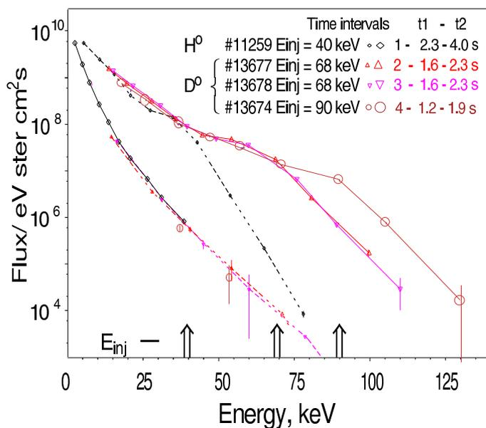
Figure 4:  $H^0$  and  $D^0$  fluxes from discharges with 40, 68, and 90 keV beam injection energy.
