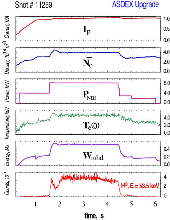
Figure 1: Improved H-Mode discharge in Hydrogen with 8.6 MW  $H^0$  Beam Injection from 8 Sources.
