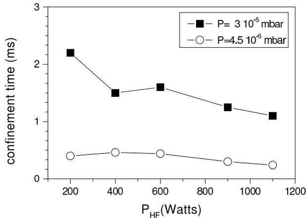
Figure 2: Electron confinement time.
