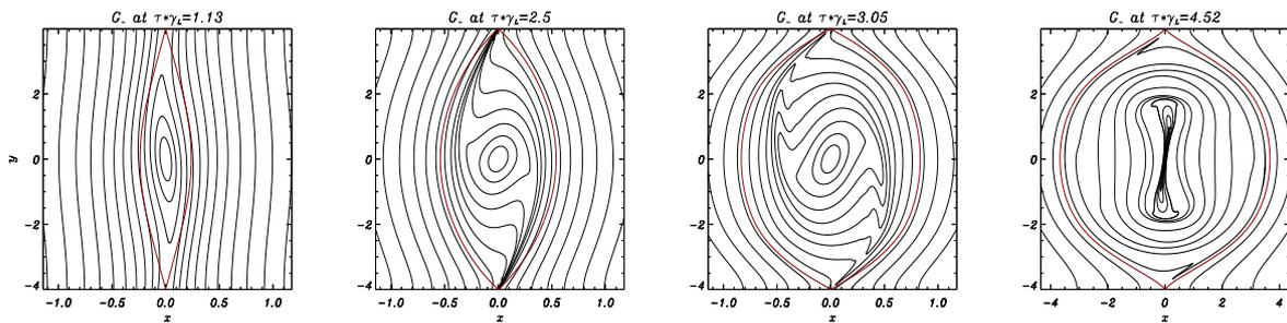
Figure 2: Contour plots of  $G_-$  at different simulation times. The separatrix of the magnetic flux,  $\psi$ , is in red
