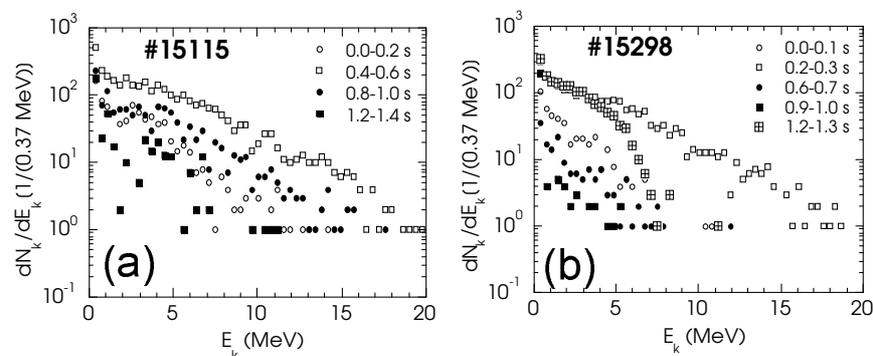
Figure 1: Bremsstrahlung gamma-ray spectra at selected time intervals for ohmic discharge # 15115 and Lower Hybrid current drive discharge # 15298 ( $dN_k/dE_k$  is the number of photon counts per energy interval and  $E_k$  the photon energy).
