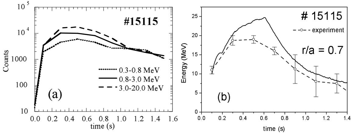
Figure 2: For ohmic discharge # 15115 ( $I_p = 700$  kA;  $B_t = 5.4$  T): (a) Time evolution of the photon counts detected by the gamma-ray spectrometer in several energy ranges; (b) Comparison between the maximum measured gamma energy (as roughly determined from the end points of the pulse height distributions) and the maximum runaway energy predicted by a test particle model of the runaway dynamics.
