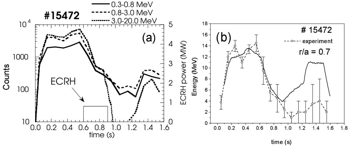
Figure 4: For ECRH discharge # 15472 ( $I_p = 400$  kA;  $P_{ECRH} = 0.8$  MW): (a) Time evolution of measured photon counts in several energy ranges; (b) Comparison between maximum measured gamma energy and maximum predicted runaway energy.
