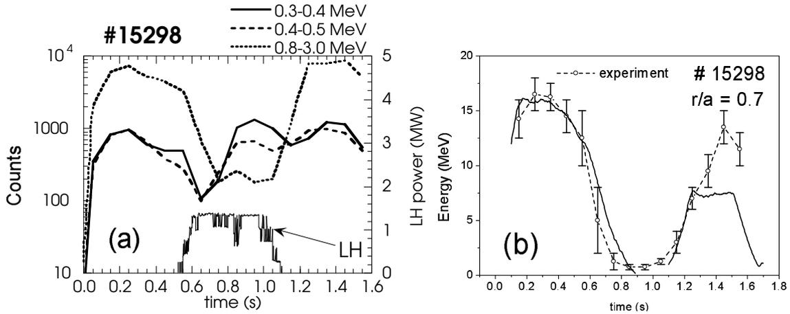
Figure 3: For Lower Hybrid current drive discharge # 15298 ( $I_p = 350$  kA;  $P_{LH} = 1.4$  MW): (a) Time evolution of the photon counts detected by the gamma-ray spectrometer in several energy ranges; (b) Comparison between maximum measured gamma energy and maximum predicted runaway energy.
