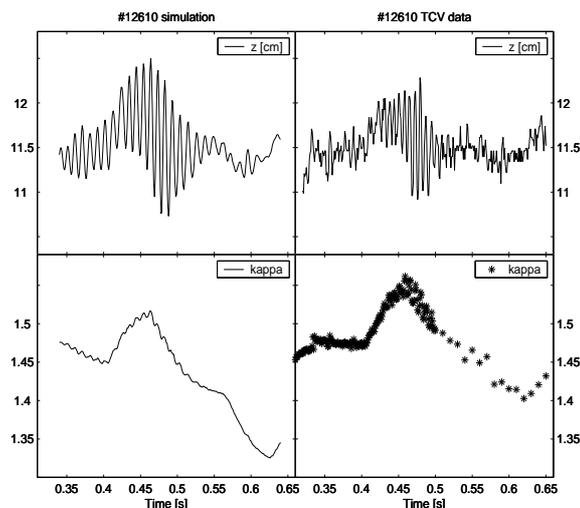
Figure 4 Comparison between TCV (left) and the DINA simulation (right) for a large excursion due to a square voltage pulse OHI stimulation. The vertical position goes closed loop unstable and returns to closed loop stable once the elongation is reduced.
