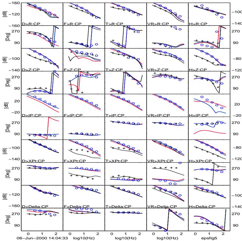
Figure 5 Selected open-loop responses from the JT-60U tokamak
