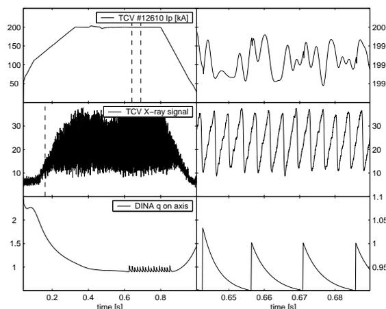
Figure 3 Comparison between DINA simulation and TCV for the evolution of the sawtooth activity: left, the full pulse showing, from top to bottom: TCV Ip, TCV soft X-ray signal, DINA  $q(0)$ ; right, an expanded view of the same signals.
