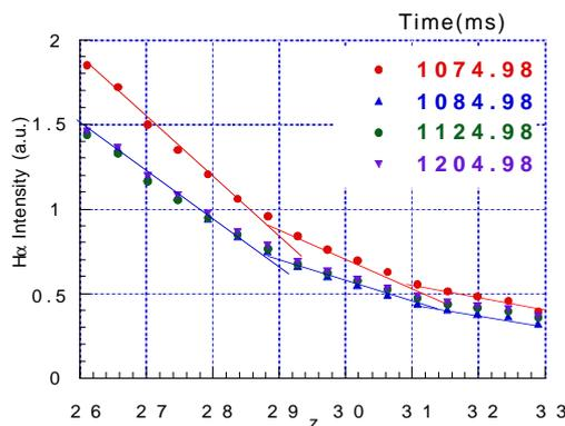
Fig.4 H $\alpha$  profiles during density ramping by external puffing( Poloidal Lim. At z=29)
