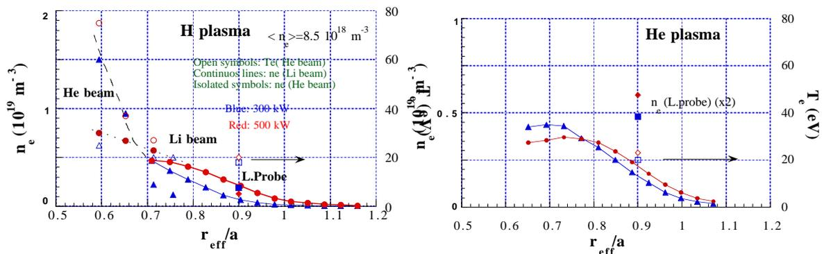
Fig. 1. Plasma edge profiles of electron density and temperature for  $\text{H}$  and  $\text{He}$  plasmas at constant density. Two cases of  $P_{in}$  (300 and 500kW) are shown for each species.
