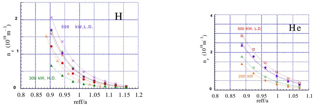
Fig.3 S.O.L density radial profiles for H and He plasmas
