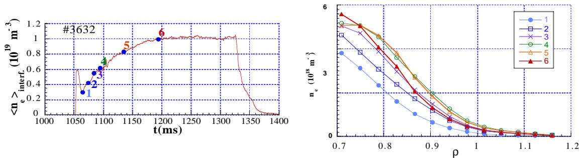
Fig 2. Time evolution of electron density profiles at the edge during density ramp-up
