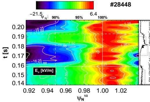
**Figure 3:** Evolution of the radial electric field for shot 28448.
