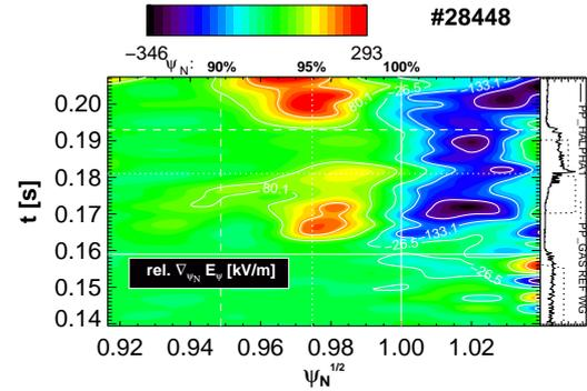
**Figure 4:** Evolution of  $\partial E_\Psi / \partial \Psi_N$  relative to the shear during the first L-mode phase for shot 28448.
