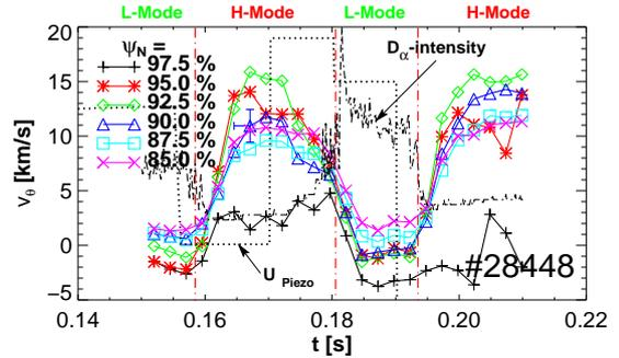
**Figure 2:** Poloidal velocity on constant flux surfaces as a function of time.
