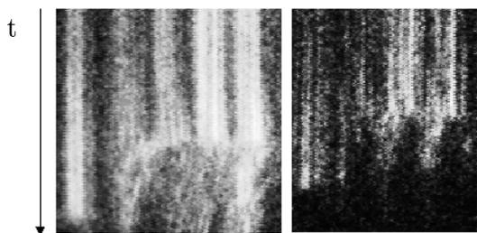
Figure 4: *Images from the VISAR : we can measure the fringe shift, get an independent measurement of the shock transit time in the Al step, and measure the reflectivity of the target.*
