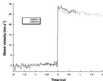
Figure 5: *Shock velocity profile measured with the VISARS from the images of fig. 4. The shock is stationnary.*
