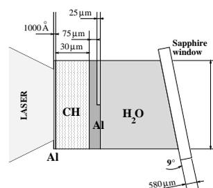
Figure 2: *Target.* The interface between Al and Water is made of a  $25 \mu\text{m}$  step.
