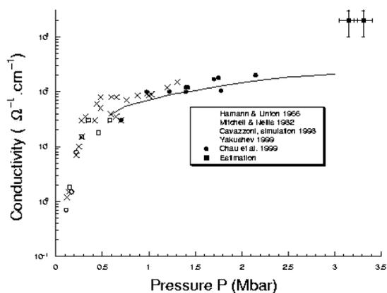
Figure 7: Estimation of the electronic conductivity and comparison with measurements [7, 10, 9]. The curve is the ab initio calculation of Cavazzoni [1]. The temperature for the two shots is about 2.6 eV.
