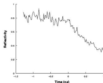
Figure 6: *Reflectivity of the target measures from the images of fig. 4. Initially, the reflecty decreases because of a small preheating of the target. It seems to stabilize further around the value 0.3.*
