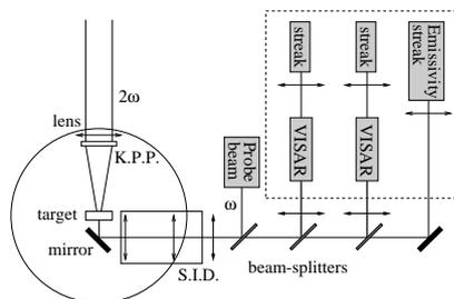
Figure 1: *Set-up.* The power laser beam ( $\lambda = 0.526 \mu\text{m}$ ) is optically smoothed by a KPP and focused on the target; a probe beam ( $\lambda = 1.064 \mu\text{m}$ ) is reflected on its rear side and analysed by two VISAR; the emissivity of the target is recorded by a third di-agnostic.
