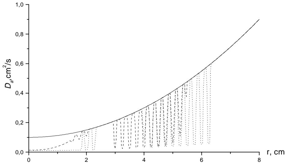
Fig.3 Anomalous diffusion coefficient (solid-29.5 ms, dashed-31 ms, dotted-33ms)
