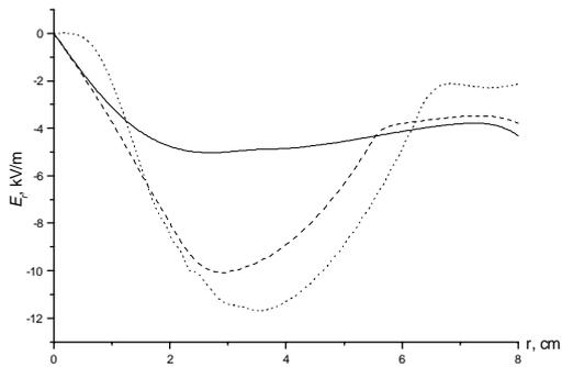
Fig.4 Radial electric field (solid-29.5 ms, dashed-31 ms, dotted-33ms)
