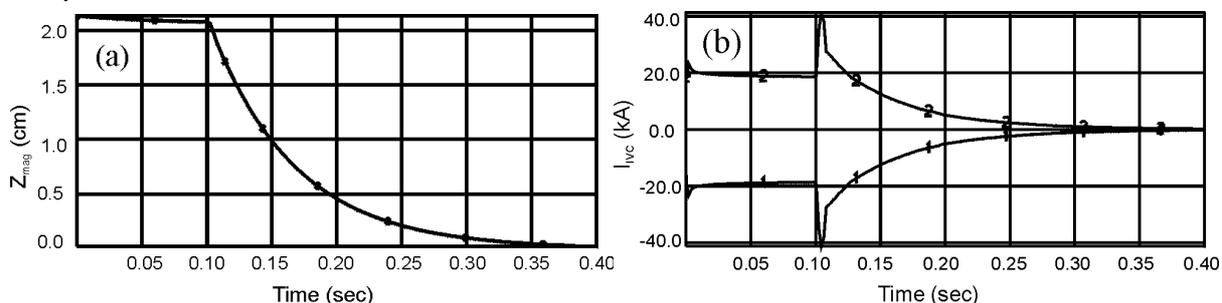
Fig 4. Time histories of (a)  $Z_{mag}$  and (b) feedback currents in IVC for 2 cm step response simulation.
