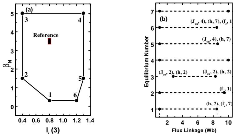
Fig 3. (a) Steady-state operating space for full-current (2 MA) KSTAR plasmas. (b) Ohmic operation window for seven equilibria.
