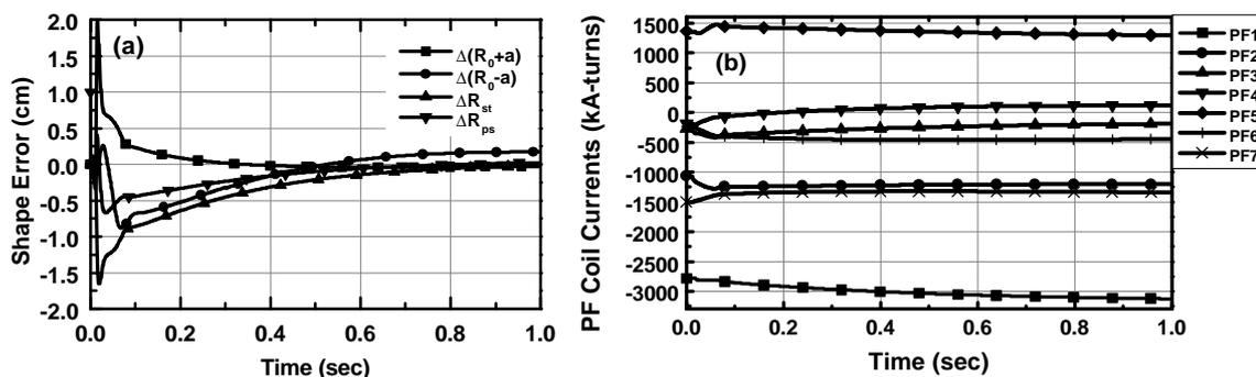
Fig 6. Time histories of (a) shape errors and (b) currents in PF coils during the shape control simulation.
