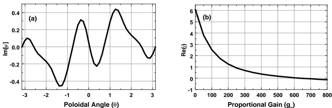
Fig 8. (a) Poloidal mode structure of  $m=2, n=1$  resistive wall mode. (b) Growth rate of resistive wall mode vs. proportional gain.
