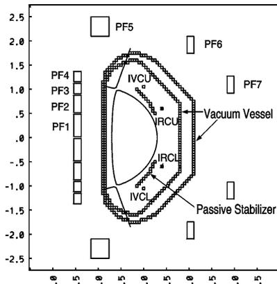
*Fig. 1. Axisymmetric model of KSTAR*
