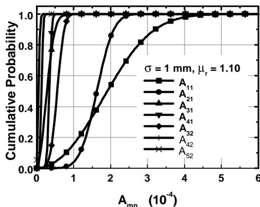
Fig 7. Cumulative probability of normalized  $(m,n)$  error field amplitude. misalignment is 1 mm. It has been shown that the maximum of 20 kA FEC/RWM coil current is required to satisfy the error field tolerance.
