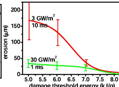
Fig. 4. Calculated brittle destruction of vertical ITER-FEAT graphite targets as function of damage threshold energy for two different off normal events.
