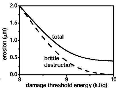
Fig. 2a. Calculated erosion for perpendicular pyrolytic graphite targets for MK-200 UG gun facility.
