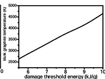
Fig. 2b. Damage threshold energy and related bulk graphite temperature.
