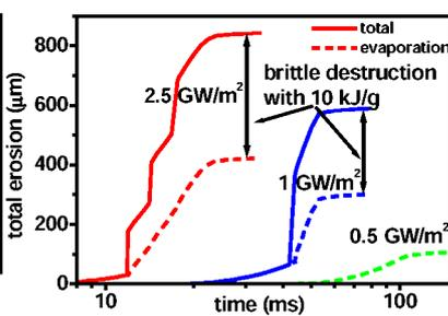
Fig. 3. Total erosion and evaporation of CFC graphite for 15 MeV runaway electrons. Target heat load is 50 MJ/m<sup>2</sup>. The inclination angle of the hot electrons is 1°.
