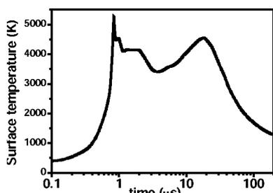
Fig. 2c. Evolution of surface temperature of a graphite target in plasma gun experiments with peak target heat load of 300 GW/m<sup>2</sup>.
