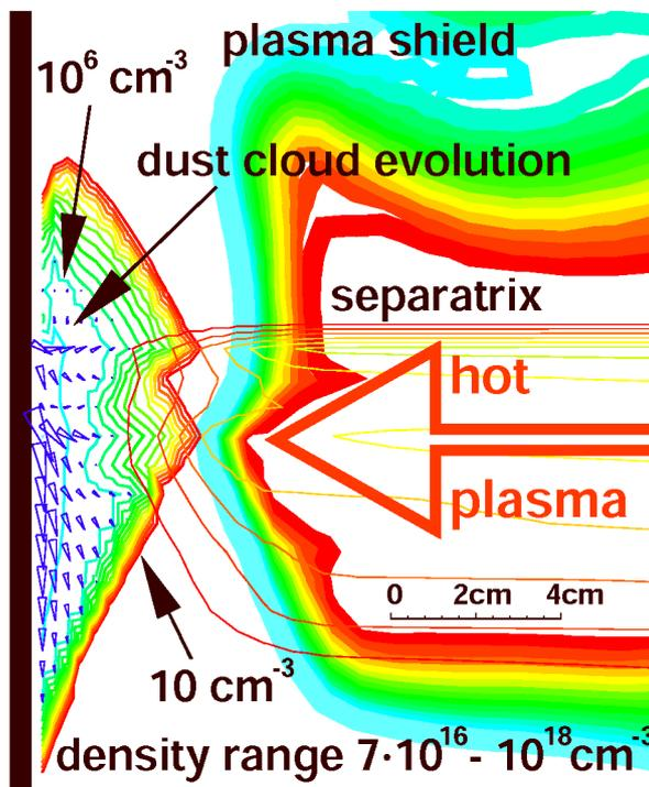
Fig. 6. Motion pattern and densities in the dust cloud and plasma shield particles at 0.4 ms.
