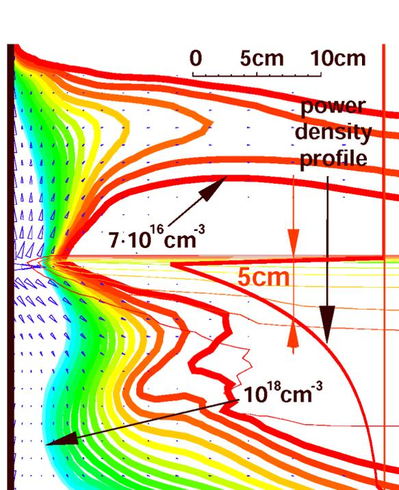
Fig. 5. Density contours and plasma flow pattern for horizontal graphite target, peak target heat load 100 GW/m<sup>2</sup> at 0.4 ms.
