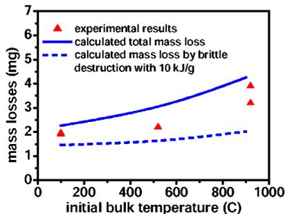
Fig. 1. Total mass loss for CFC graphite for JEBIS conditions with 70 keV e-beam, pulse duration 2 ms, absorbed heat flux 1.8 GW/m<sup>2</sup>.
