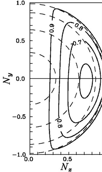
Fig.3. 2D representation of the reflection coefficient for O mode (standard case).
