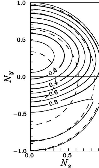
Fig.4. 2D representation of the reflection coefficient for X mode (standard case).
