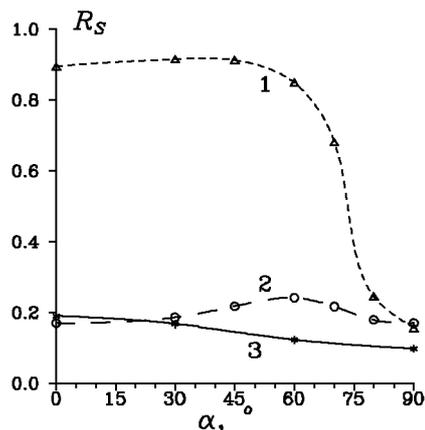
Fig.5. Reflection coefficient of 2 waveguide antenna versus angle of rotation  $\alpha$  for different central densities (see text).
