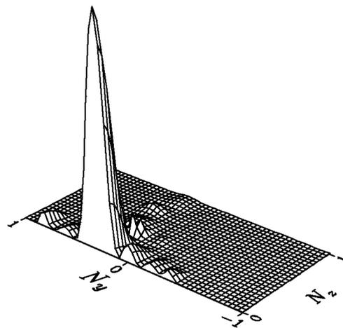
Fig.6. 2D spectrum excited by  $4 \times 12$  waveguide antenna at  $\alpha = 0^\circ$ .
