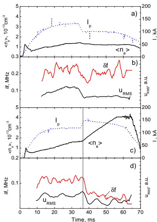
Fig.1 Comparison of waveforms for the current ramp down b) and up d) experiments. Vertical line marks the moment of the transitions. a), c) – plasma current and density for CRD and CRU respectively. O –mode, b) -  $F=18$ GHz, d) -  $F=22$ GHz
