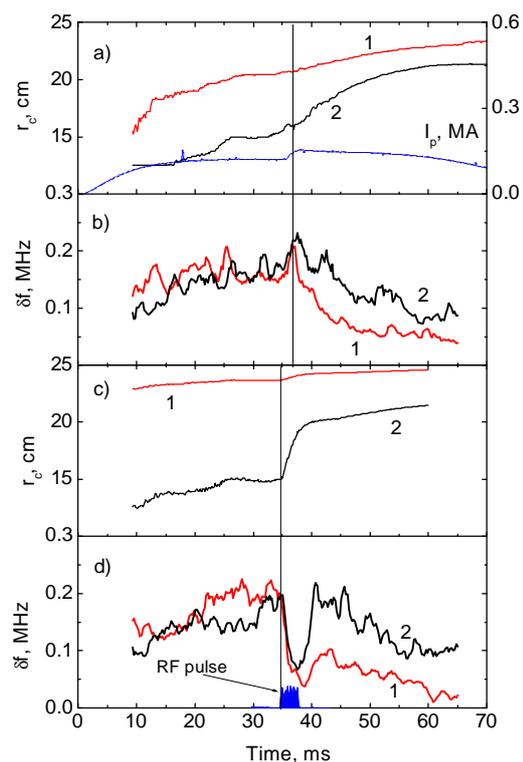
Fig.4 Comparison of spectrum width for various cut of layer position (a, c) under CRU (a, b) and ICRH (c, d) H-mode initiations. O – mode, 1 –  $F=17.5GHz$ , 2 –  $F=25GHz$
