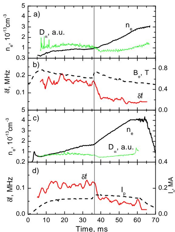
Fig.2 Comparison of spectrum width behavior for magnetic compression (a, b) and CRU triggering (c, d). O-mode, b) –  $F=17.5$  GHz, d) –  $F=18$  GHz
