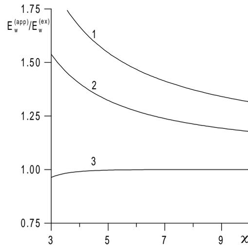
Fig. 1. Ratio of approximate values of the electric field at the surface given by different models to the exact value. 1: Child-Langmuir model. 2: ion layer-quasineutral plasma model. 3: exponential-accuracy model.
