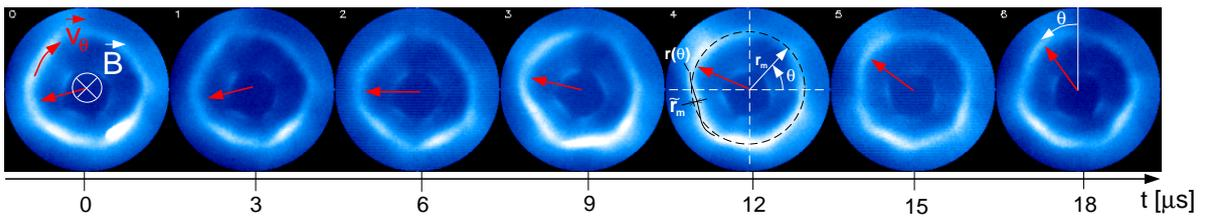
Fig. 5: Sequence of CCD-images of the plasma cross-section in the full visible spectral range. The directions of the rotation of the IDW, the electrons and the ions are identical, and are right-handed to  $\vec{B}$ , due to the  $\vec{E} \times \vec{B}$ -motion with  $E_r < 0$  at the position of the inboard IDW.
