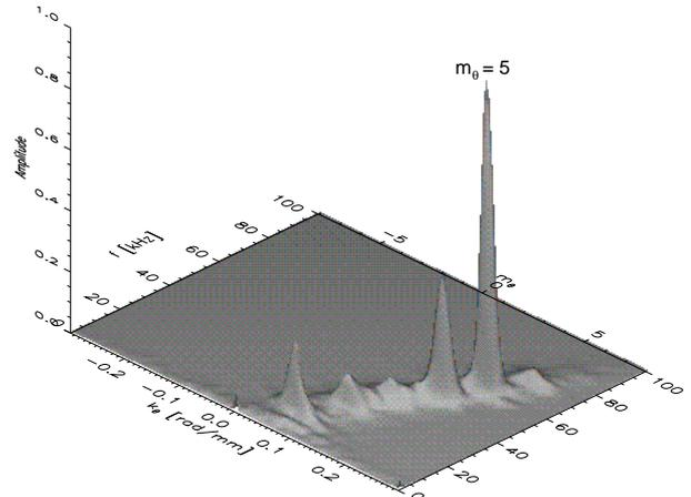
Fig. 4: Wavenumber-frequency-spectrum of  $U_{f1}$  (azim. dispersion-relation of the inboard IDW).
