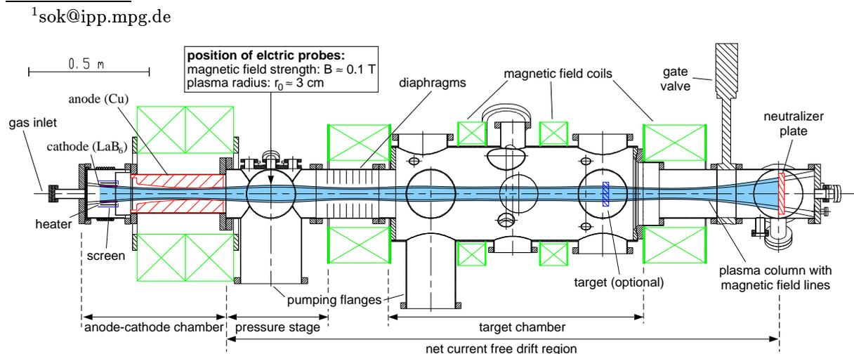
*Fig. 1: The Plasma-Generator PSI-2.*
