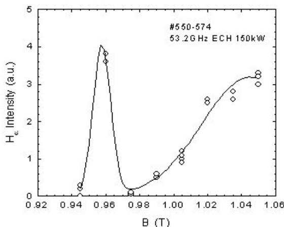
Fig. 6 Dependence of  $H_{\alpha}$  emission on magnetic field strength. The field configuration is kept constant.
