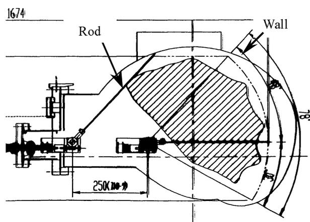
Fig. 3 Fluorescent rod scanning system. The shaded area is the outermost magnetic surface in the standard configuration.
