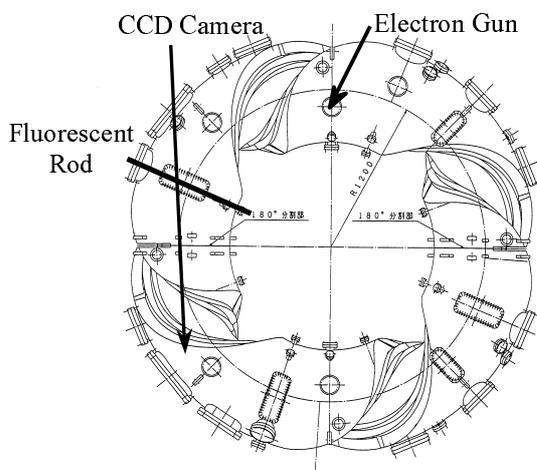
Fig. 2 Experimental Setup for Vacuum Magnetic Surface Mapping.
