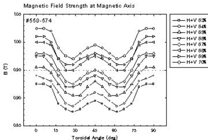
Fig. 7 Magnetic field strength on the magnetic axis in the toroidal direction. The field strength is scanned with the field configuration kept constant.
