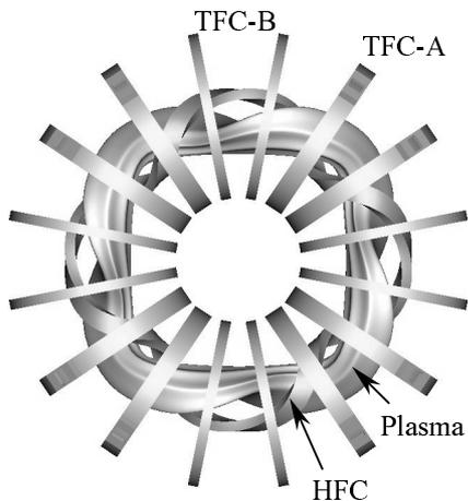
Fig. 1 A schematic view of the Heliotron J device.
