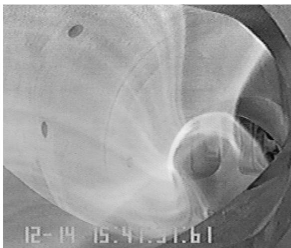
Fig. 5 A tangential view of ECH plasma measured with a CCD camera.
