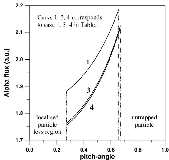
Fig.3. Calculated pitch-angle dependence of the alpha loss flux to the first wall in the plasma midplane for different plasma shapes.
