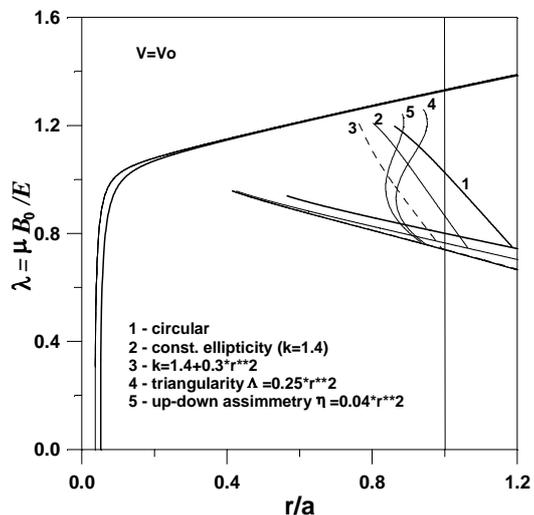
Fig.1a. Curves 1-5 represent the solution of Eq.(3) in the phase space for different FS shapes. The upper curve corresponds to the boundary of the confinement domain of co-moving particles.
