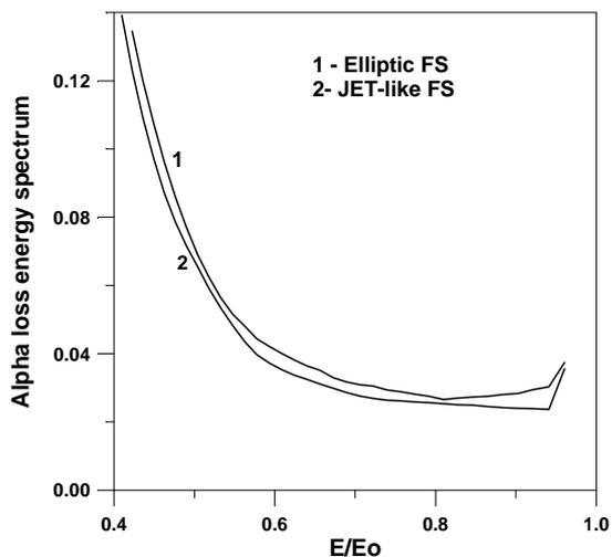
Fig.2. Calculated alpha loss energy spectrum vs. particle energy for different plasma shapes.  $E_0$  is the alpha birth energy.
