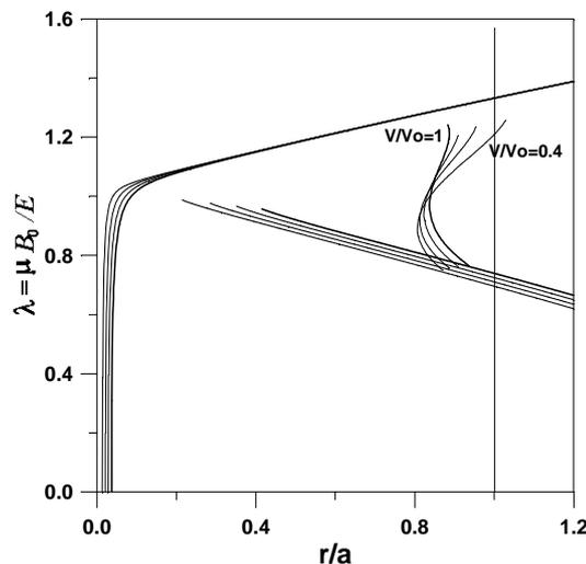
Fig.1b. Energy dependence ( $V_0$ =birth velocity) of the stochasticity threshold for the case of a JET-like flux surface configuration. The vertical line corresponds to the radius of the last closed surface.
