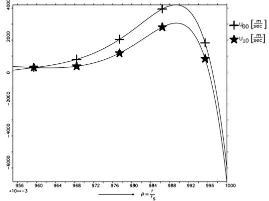
Figure 2:  $U_{\perp 0}$  [m/sec] and  $U_{\theta 0}$  [m/sec] inside the separatrix for normal  $\vec{B}$  direction
