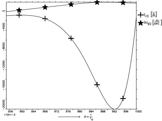
Figure 3:  $E_{r0}$  [V/m] and  $\Theta U_{\parallel 0}$  [m/sec] inside the separatrix for inverted  $\vec{B}$  direction
