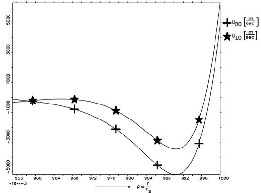
Figure 4:  $U_{\perp 0}$  [m/sec] and  $U_{\theta 0}$  [m/sec] inside the separatrix for inverted  $\vec{B}$  direction
