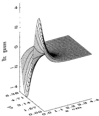
Fig. 4 Space-time profile of the wave magnetic field  $B_z$ .
