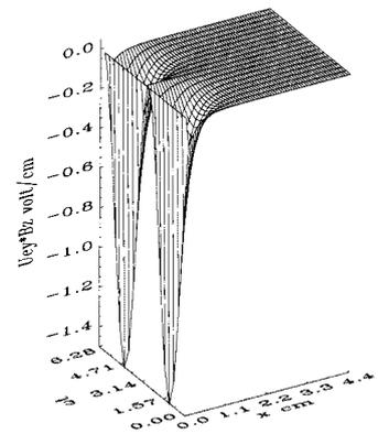
Fig. 6 Space-time profile of the force term  $u_{ye} B_z$ .
