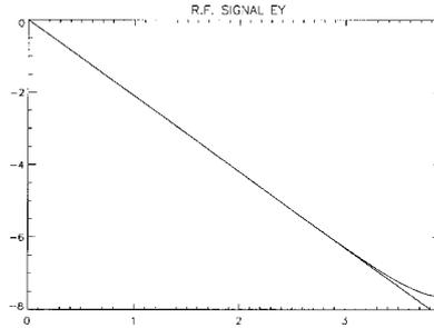
Fig. 2 The amplitude of the transverse electric field closely matches a simple exponential with scale length  $\delta = c / \omega_{pe}$ .
