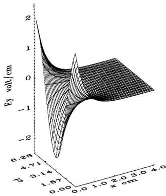
Fig. 1 Space-time profile of the transverse electric field  $E_y$ .
