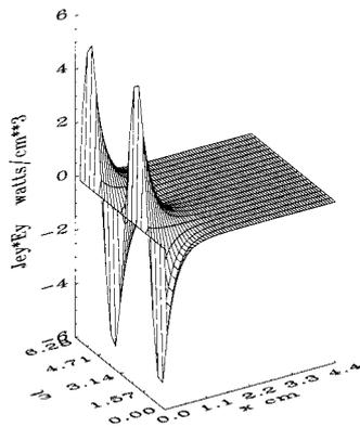
Fig. 5 Space-time profile of the heating term  $j_y E_y$ .
