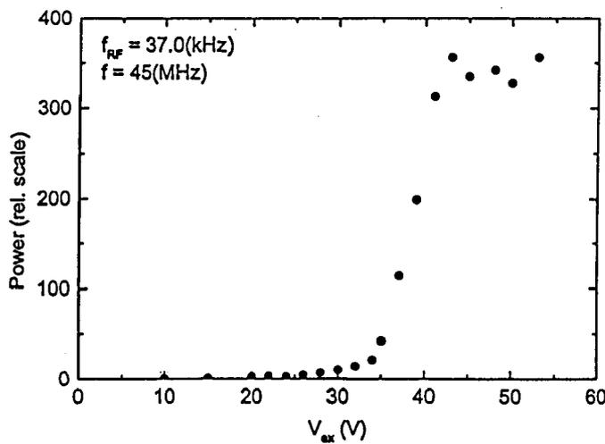
[Fig.4] Relation of HF power with LF amplitude  $V_{ex}$ .
