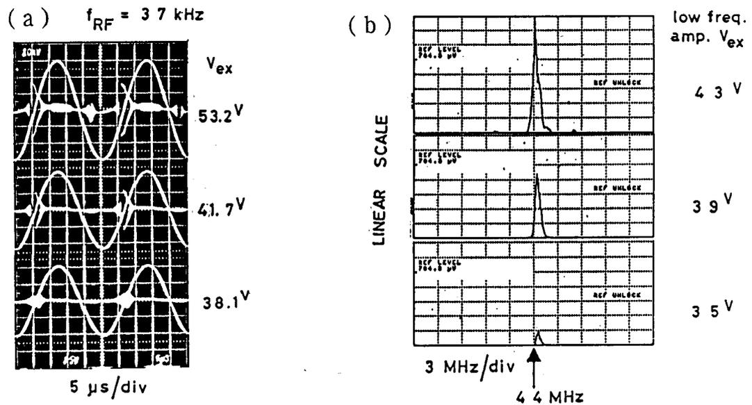
[Fig.3] (a) HF signals controlled by applied LF fields with amplitudes  $V_{ex}$ . (b) Spectra of HF oscillations changing with  $V_{ex}$ .
