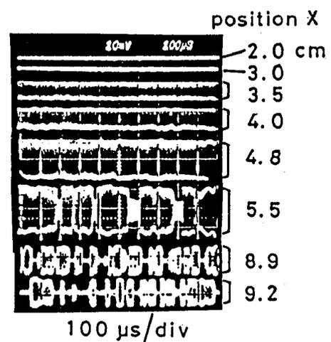
[Fig.2] Oscilloscope traces of HF oscillation signals observed at various  $x$ . ( $f_{HF} = 40-45 \text{ MHz}$ )
