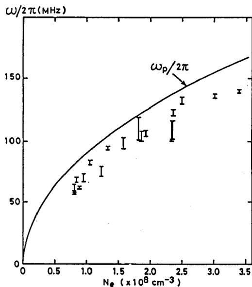
[Fig.1] Relation of HF oscillation frequency with plasma density.
