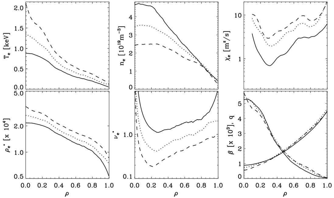
Figure 3: Profiles of RTP discharges r19971119.062 (I,full), -058 (dotted), and -051 (II,dashed). Plasma parameters:  $B = 2.00 - 2.02 T$ ,  $I_p = 82$  kA,  $P_{ECH} = 40, 200, 305$  kW, respectively.
