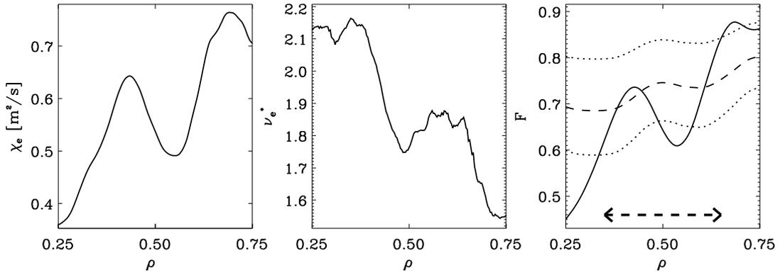
Figure 2: Quotients  $\chi_I/\chi_{II}$ ,  $\nu^*_I/\nu^*_{II}$  and  $F_I/F_{II}$  for discharges I and II of Fig.1 (full lines). In the right panel also  $(\nu^*_I/\nu^*_{II})^\zeta$  for  $\zeta = -0.3, -0.5$  and  $-0.7$  (dotted/dashed/dotted line).
