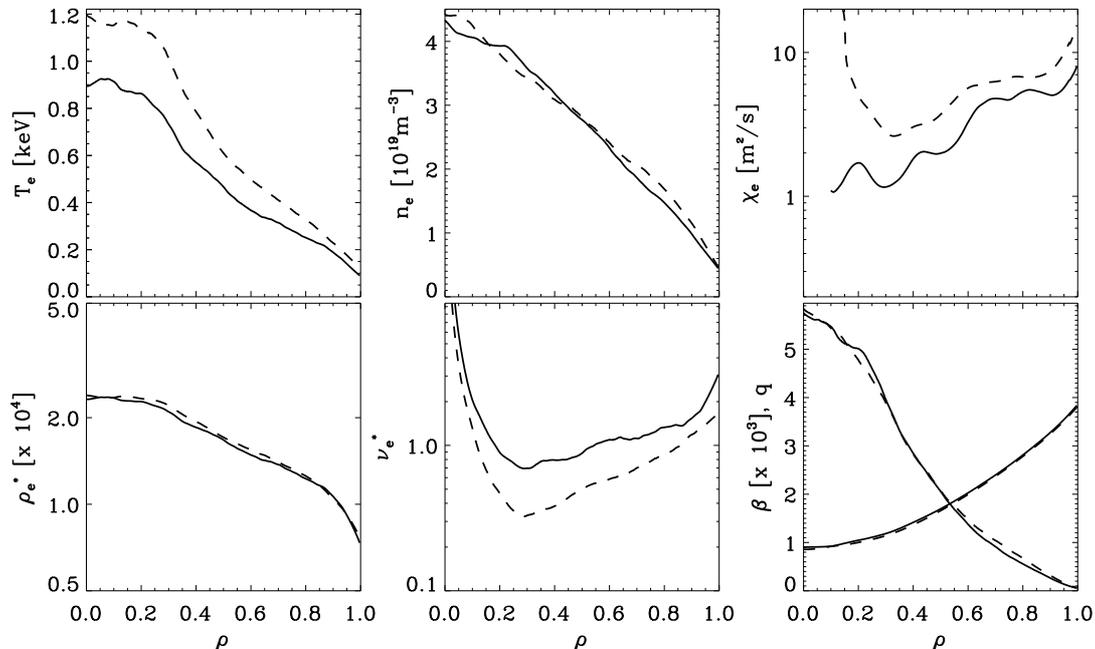
Figure 1: Profiles of RTP discharges r19971119.073/068 (I/II, full/dashed lines). Plasma parameters:  $B = 1.88/2.10$  T,  $I_p = 91/103$  kA,  $P_{ECH} = 90/310$  kW, respectively.
