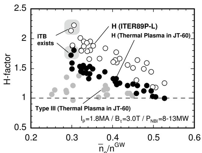
Fig.1  $H$ -factors for ELMy H-mode discharges in JT-60U as a function of  $\bar{n}_e / n^{GW}$
