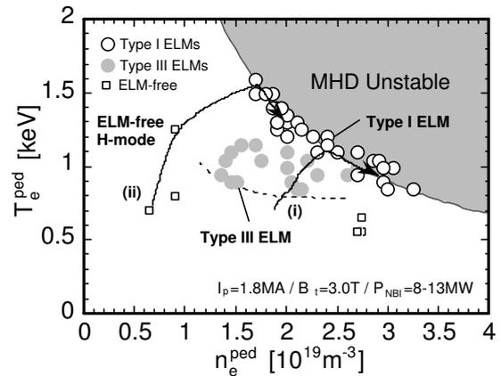
**Fig.5** Diagram of  $n_e^{\text{ped}} - T_e^{\text{ped}}$  for classifying ELM behavior in JT-60U.
