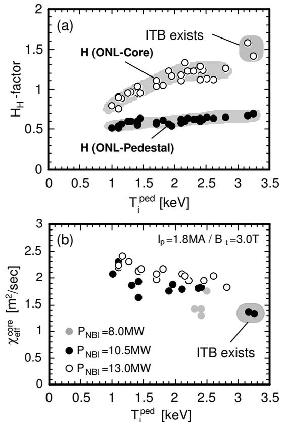
**Fig.6** Dependences of (a)  $H$  (ONL-Core),  $H$  (ONL-Pedestal) and (b)  $\chi_{\text{eff}}^{\text{core}}$  on  $T_i^{\text{ped}}$  in type-I ELMy H-mode plasmas.
