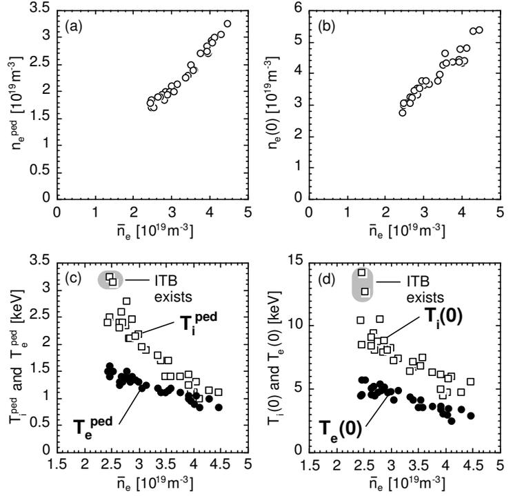
**Fig.2** Density dependences of (a)  $n_e^{ped}$ , (b)  $n_e(0)$ , (c)  $T_e^{ped}$  (closed circles),  $T_i^{ped}$  (open squares) (d)  $T_e(0)$  (closed circles) and  $T_i(0)$  (open squares) in type-I ELMy phase.
