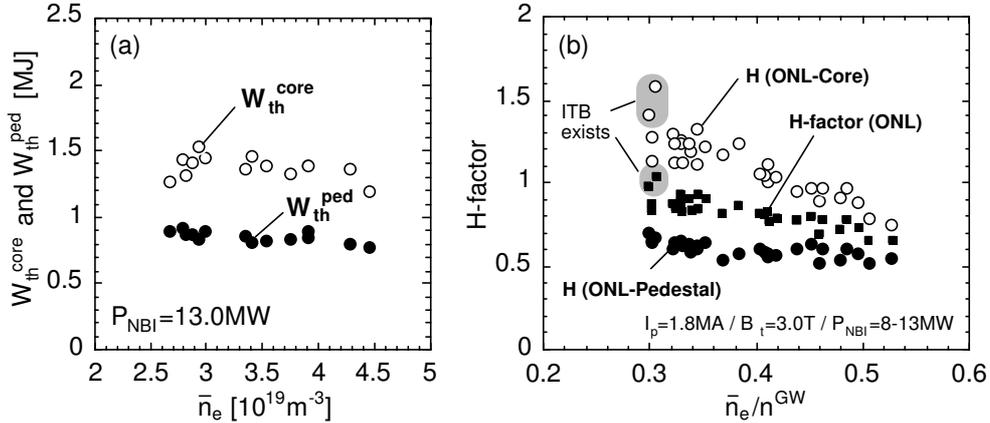
**Fig.3** (a) Density dependences of  $W_{th}^{core}$  and  $W_{th}^{ped}$  with  $P_{NBI} = 13.0 \text{ MW}$ . (b) H-factor in type-I ELMy phase based on the offset nonlinear scaling.
