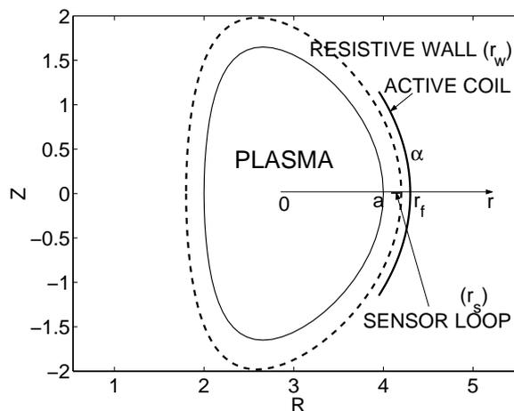
Figure 1: *Geometry of feedback control.*
