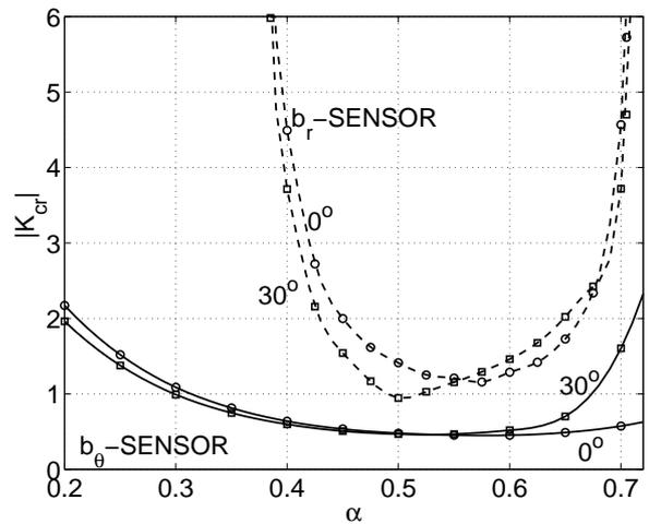
Figure 3: Magnitude of the critical gain  $|K_{cr}|$  versus the active coil width for the  $b_r$ -sensor (dashed lines) and  $b_\theta$ -sensor (solid lines) feedback schemes.
