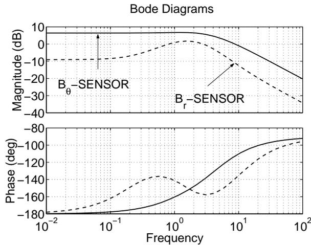
Figure 2: Bode plots of typical open loop transfer functions  $P_1^r(s)$  and  $P_1^\theta(s)$  for  $b_r$  and  $b_\theta$  sensors. The same equilibrium and feedback configuration are used as in Fig. 2.
