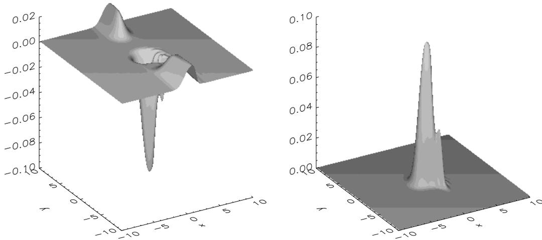
Fig. 2. Generalized potential vorticity (left) and normalized electron pressure (right) at time 800. Plasma parameters:  $d_e = 1.0$ ,  $\lambda = 0.01$ ,  $\kappa_n = 0.1$ ,  $b_y = 0.01$ , source amplitude  $S_0 = 0.001$ , source switched off at time  $t_s = 100$ .
