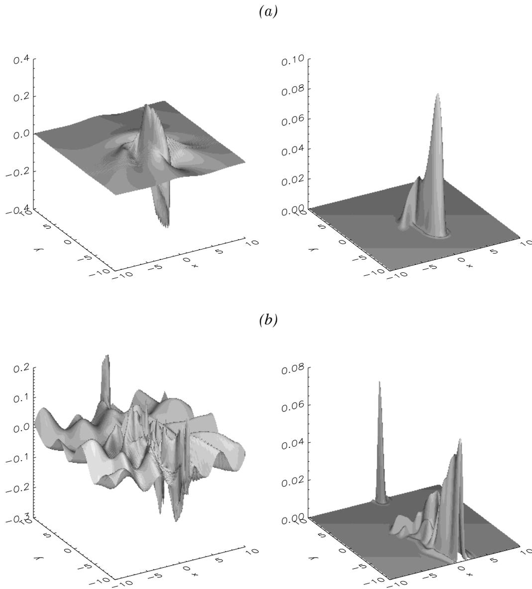
Fig. 4. Generalized potential vorticity (left) and normalized electron pressure (right) at times (a) 250 and (b) 800. Plasma parameters:  $d_e = 1.0$ ,  $\lambda = 1.0$ ,  $\kappa_n = 0.1$ ,  $b_y = 0.01$ , source amplitude  $S_0 = 0.001$ , source switched off at time  $t_s = 100$ .
