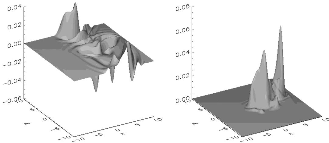
Fig. 3. Generalized potential vorticity (left) and normalized electron pressure (right) at time 140. Plasma parameters:  $d_e = 1.0$ ,  $\lambda = 0.01$ ,  $\kappa_n = 0.01$ ,  $b_y = 0.01$ , source amplitude  $S_0 = 0.001$ , source switched off at time  $t_s = 100$ .
