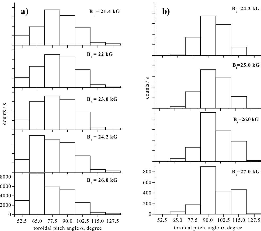
Fig. 5. Pitch-angle distributions obtained at different toroidal fields (ohmic regime,  $I_p = 320$  kA,  $\langle n_e \rangle = 4.0 \cdot 10^{13} \text{ cm}^{-3}$ , slot collimators): a) slot collimators, b) pipes collimators.
