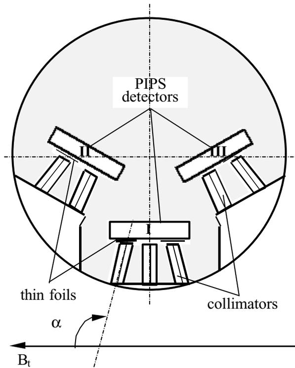
Fig. 1. Detector head (cross section).
