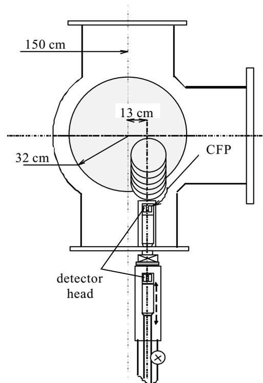
Fig. 4. T-10 CFP diagnostics (schematic view).
