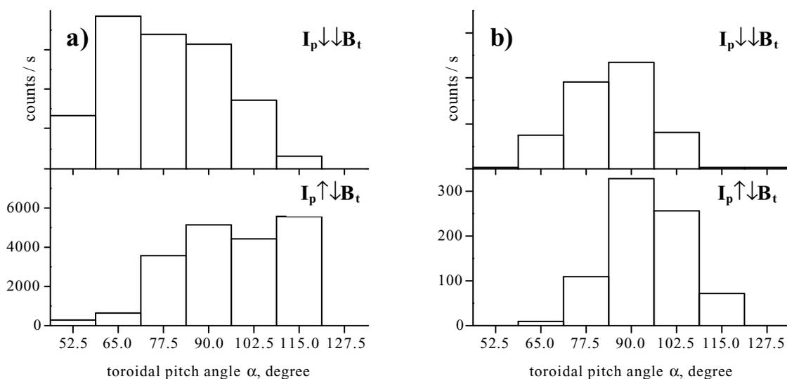
Fig. 6. Pitch-angle distributions obtained at different directions of plasma current (ohmic regime,  $B_t = 24.2$  kG,  $I_p = 300$  kA,  $\langle n_e \rangle = 3.1 \cdot 10^{13} \text{ cm}^{-3}$ ): a) slot collimators, b) pipes collimators.
