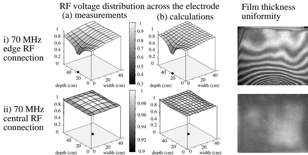
Figure 2: Measured and calculated interelectrode RF voltage distribution at 70 MHz for the edge and the central RF connection cases. The black point indicates the position of the RF and ground connections. The film interferograms show the uniformity of the film thickness for each case.
