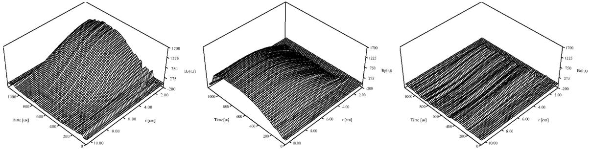
Fig.3 Time progress of each magnetic field component  $B_z$ ,  $B_p$ ,  $B_r$ .
