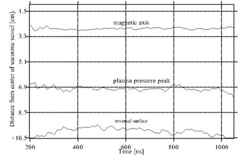
Fig.4 Time progress for the positions of magnetic axis, reversal surface and maximum pressure.
