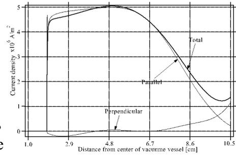
Fig.8 Profiles of total, parallel and perpendicular current densities.
