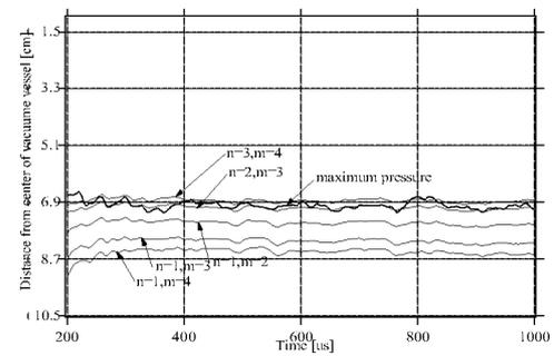
Fig.9 Positions of rational surfaces compared with the position of maximum pressure.
