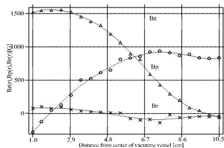
*Fig.2 Approximated radial distribution of magnetic field component.*
