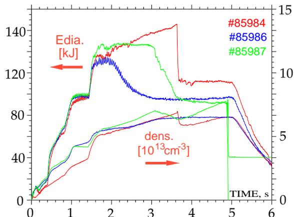
Fig.5. Variation of diamagnetic energy and density for three different gas puff scenarii.
