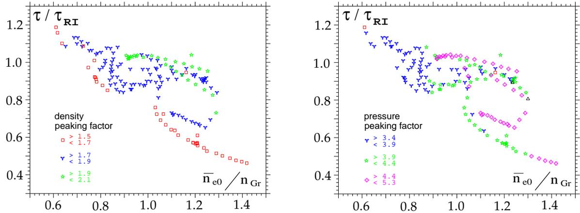
Fig. 2, 3. Confinement time respect to the RI-mode scaling versus Greenwald number with density and pressure peaking factors as parameters.
