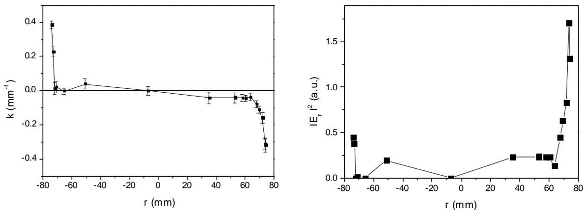
Fig. 5: Mean wave number (left) and electric energy density (right) vs. plasma radius
