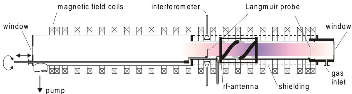
*Fig. 1 : Experimental set-up of HE-L*
