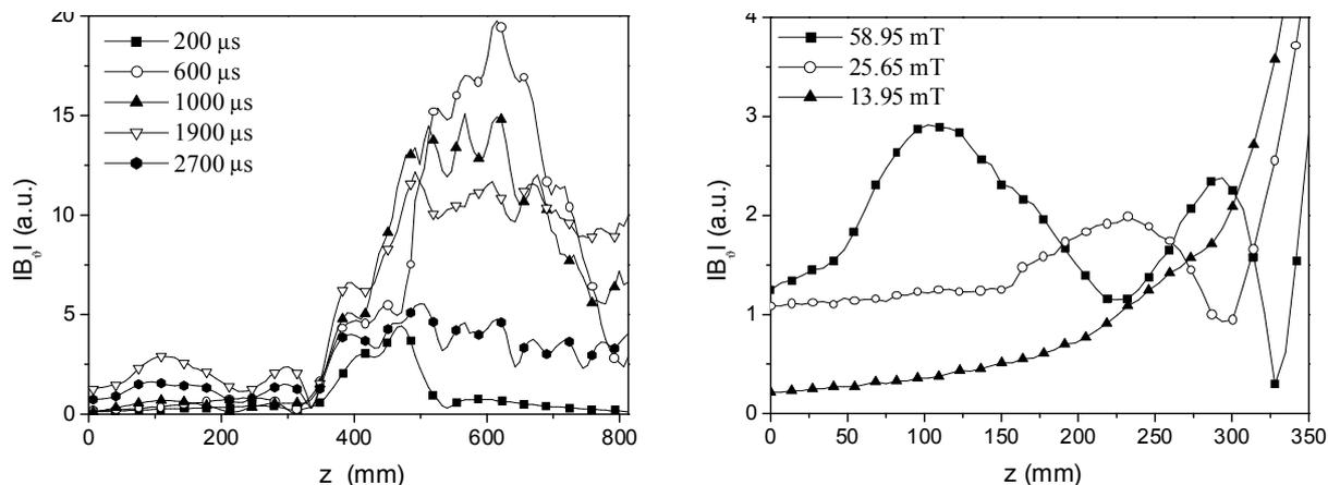
Fig.4 Axial profiles of the rf amplitude ( $B_0$ )
