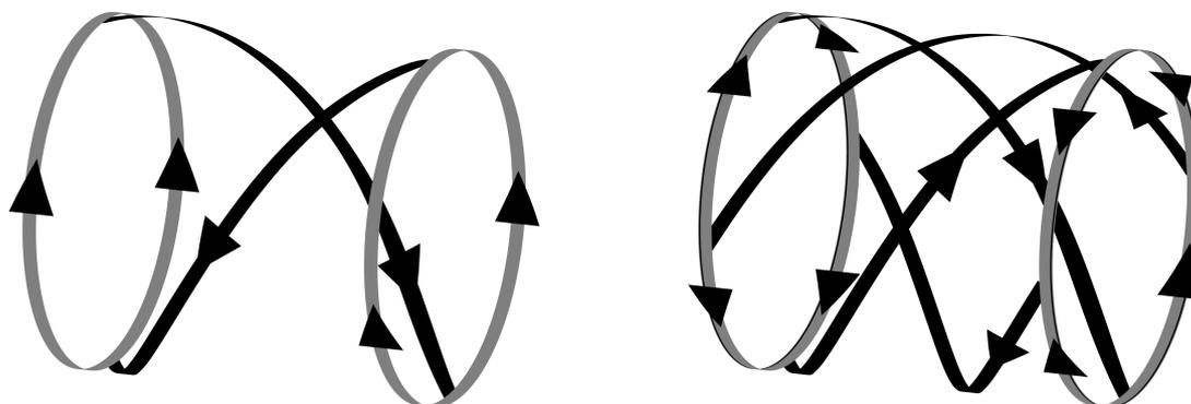
Fig. 1 : Helical  $m = 1$  (left) and  $m = 2$  (right) antennas
