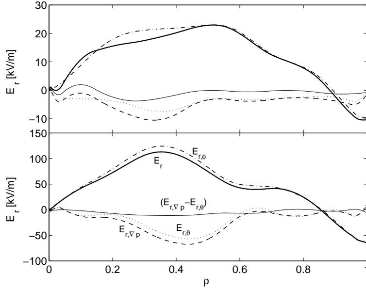
Figure 1:  $E_r$  and its components 0.6 s before (above) and 0.6 s after (below) the ITB formation for JET pulse No. 46664.
