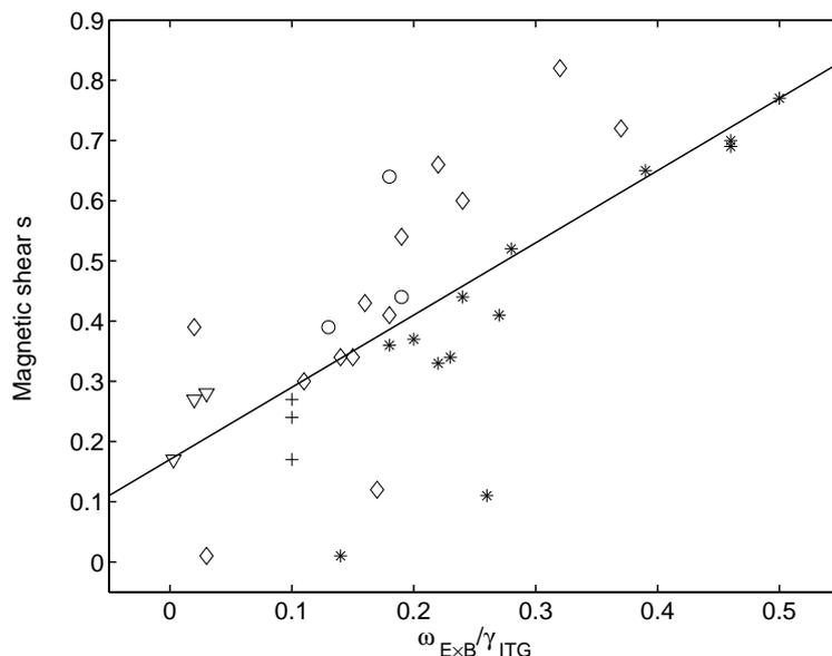
Figure 2: Magnetic shear and  $\Omega$  at the ITB location for threshold conditions. The solid line,  $s = 1.2\Omega + 0.17$  divides the region into two parts, one (upper) where an ITB does not exist and one (lower) where an ITB does exist.
