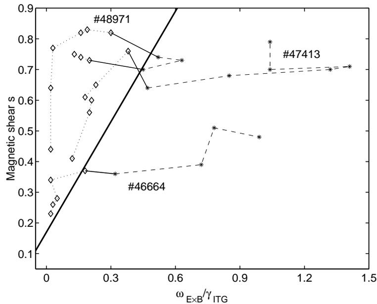
Figure 3: The time evolution of the magnetic shear and  $\Omega$  for 3 OS discharges. The same solid line,  $s = 1.2\Omega + 0.17$ , as in Fig. 2 is shown.
