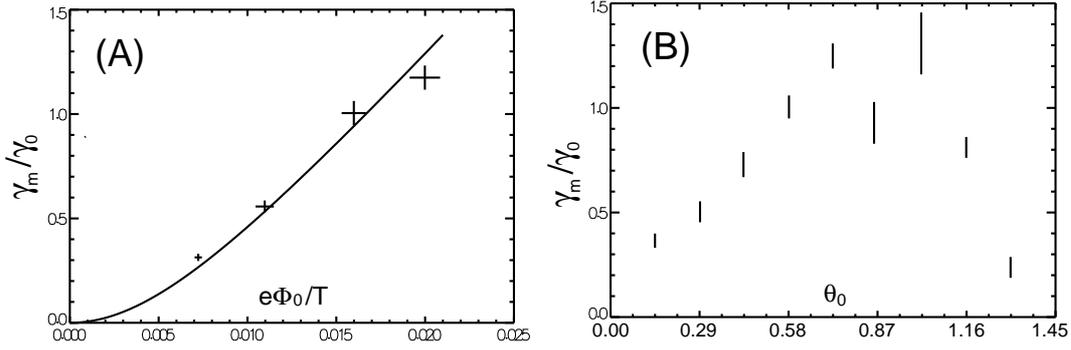
Figure 1: Gyrokinetic simulation results of zonal flow growth rate (A) vs. ITG mode amplitude for fixed  $\theta_0$ , and (B) vs.  $\theta_0$  for fixed ITG amplitude, normalized to ITG growth,  $\gamma_0$ . The line in (A) is the solution of Eq. 3.
