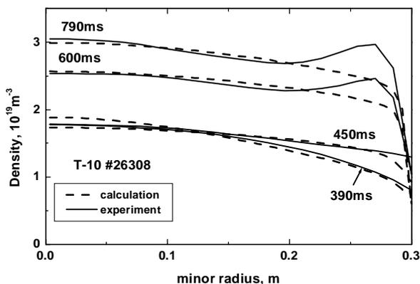
Fig.3. Experimental and calculated density profiles in T-10.
