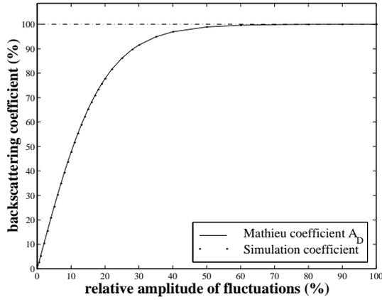
Fig.2 Back-scattering of a wave train according to the relative amplitude of the density fluctuations
