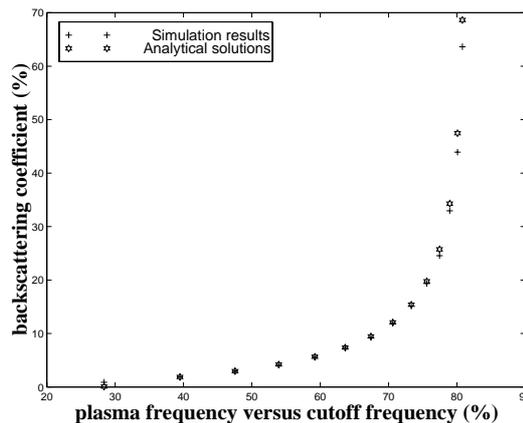
Fig.5: Back-scattering in an inhomogeneous plasma perturbed by density fluctuations
