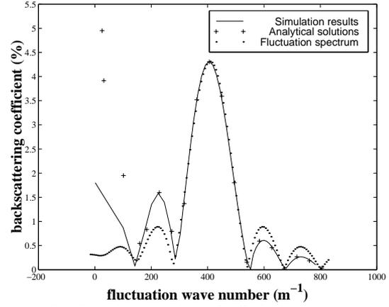
Fig.3 Fluctuation spectral effects on the back-scattered wave during frequency sweep
