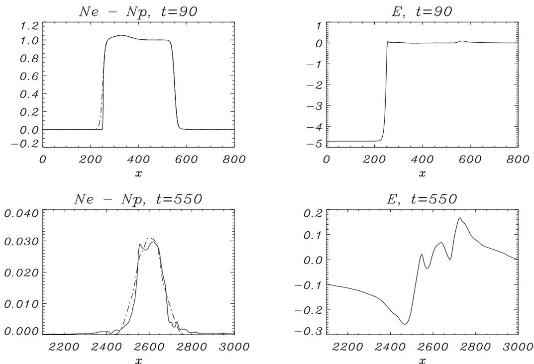
Figure 1: Interaction of a non compensated proton beam with a plasma foil. The electron and proton densities (continuous and dash-dotted lines) and the electric field at  $t = 90$  for  $0 < x < 800$  (upper frames) and at  $t = 550$  for  $2100 < x < 3000$  (lower frames).
