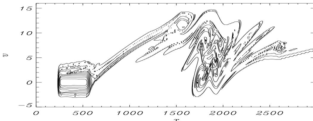
Figure 2: The electron distribution in phase space at  $t = 425$  in the case of a non compensated proton beam interacting with a plasma foil.
