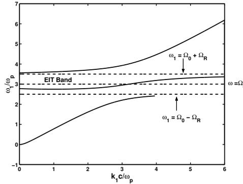
Figure 3: EIT dispersion curve,  $\Omega_0/\omega_p = 3$  and  $\Omega_R/\omega_p = 1/2$ . Flat band above  $\Omega_0 - \Omega_R$  up to  $\Omega_0 + \Omega_R$  labelled “EIT Band” corresponds to “slow light” in the presence of a pump.
